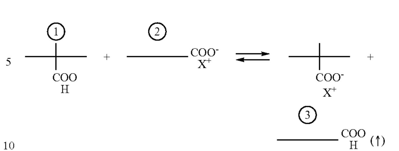
(1) un-neutralized acid group present on the ionomer resin
