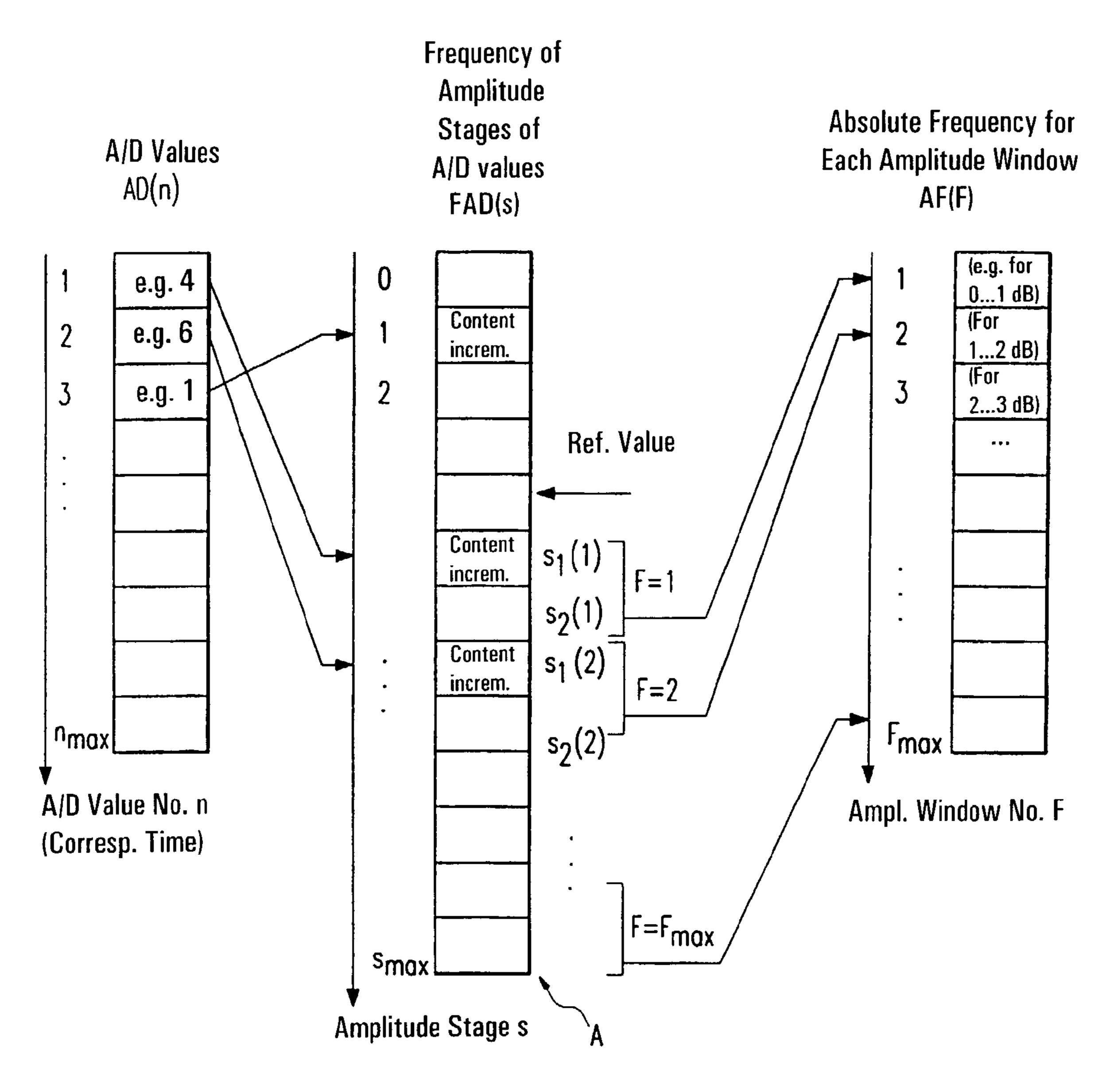
Calculation of amplitude distribution, reference value and crest factor:
