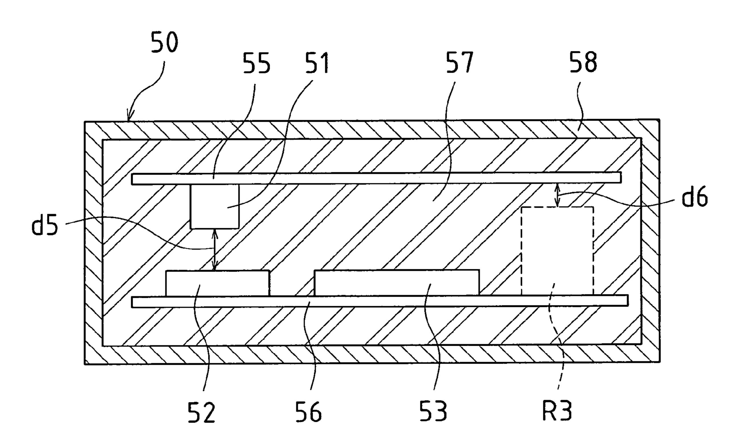
SOLID STATE RELAY, ELECTRONIC DEVICE, AND METHOD FOR MANUFACTURING SOLID STATE RELAYS HAVING A FIRST CONTROL TERMINAL, A FIRST OUTPUT TERMINAL AND A SECOND **OUTPUT TERMINAL AS LEAD TERMINALS**
