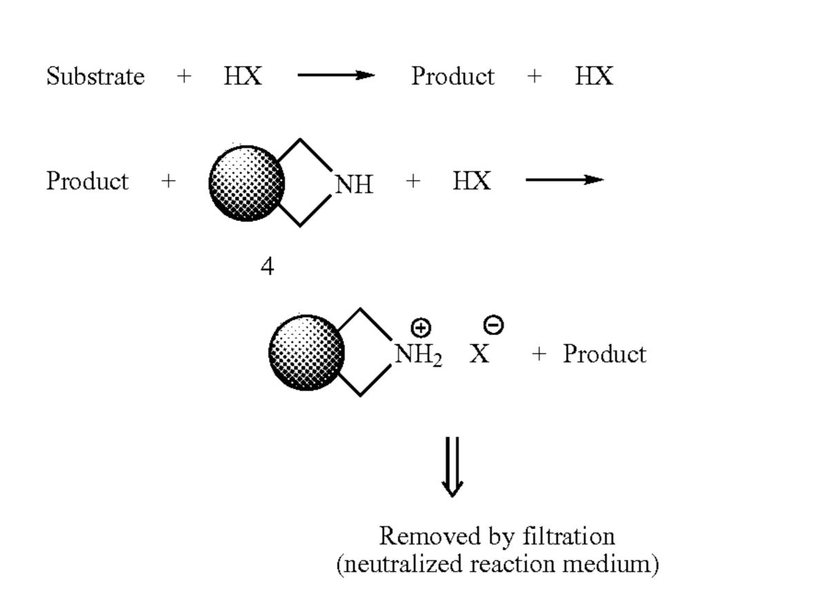
As the polyimine is amphiphilic, it can be used to trap inorganic acids in the aqueous phase as in the organic phase. Thus, the reaction medium comprising the desired product is neutralized and freed from neutralization salts by simple filtration. This facilitates is the isolation of the desired product insofar as stages of extraction at different pH values are avoided.
