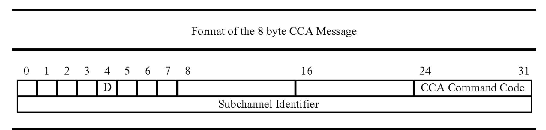
As an example, when the IOP needs to process a SSCH instruction that was issued by a program running on a CP, as part of that processing, the IOP will need to send a CCA message to a selected channel to process the SSCH for the subchannel (SCB) specified by the program. Note that an 5 SCB is a control block in HSA that contains the controls for managing an I/O operation for a specific device.
