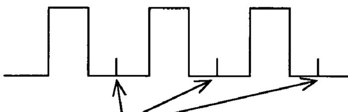
Pilot signal is output during Off
