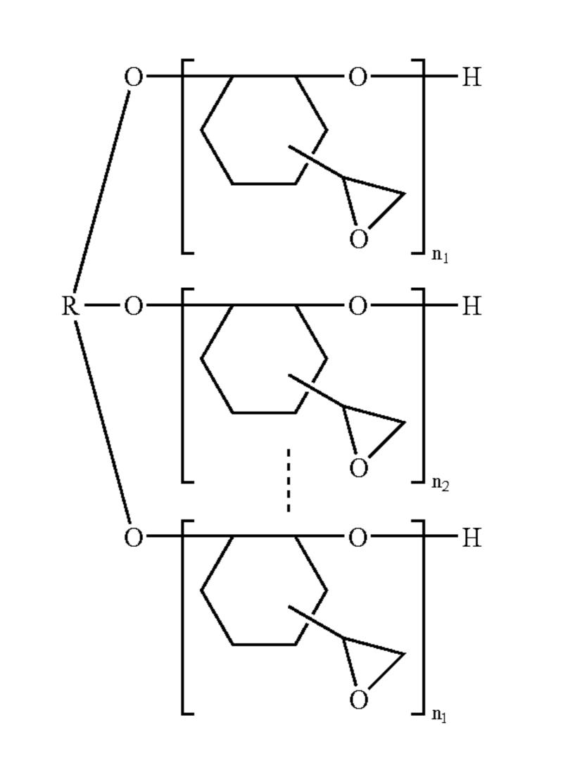
wherein R is a hydrocarbyl group and n<sub>1</sub> through n<sub>2</sub> each represent 0 or an integer of from 1 to 100 and the sum of the integers represented by n<sub>1</sub> through n<sub>2</sub> is from 1 to 100. Suitable oxirane resins of formula I may be made following the procedures disclosed in U.S. Pat. No. 4,565,859.
