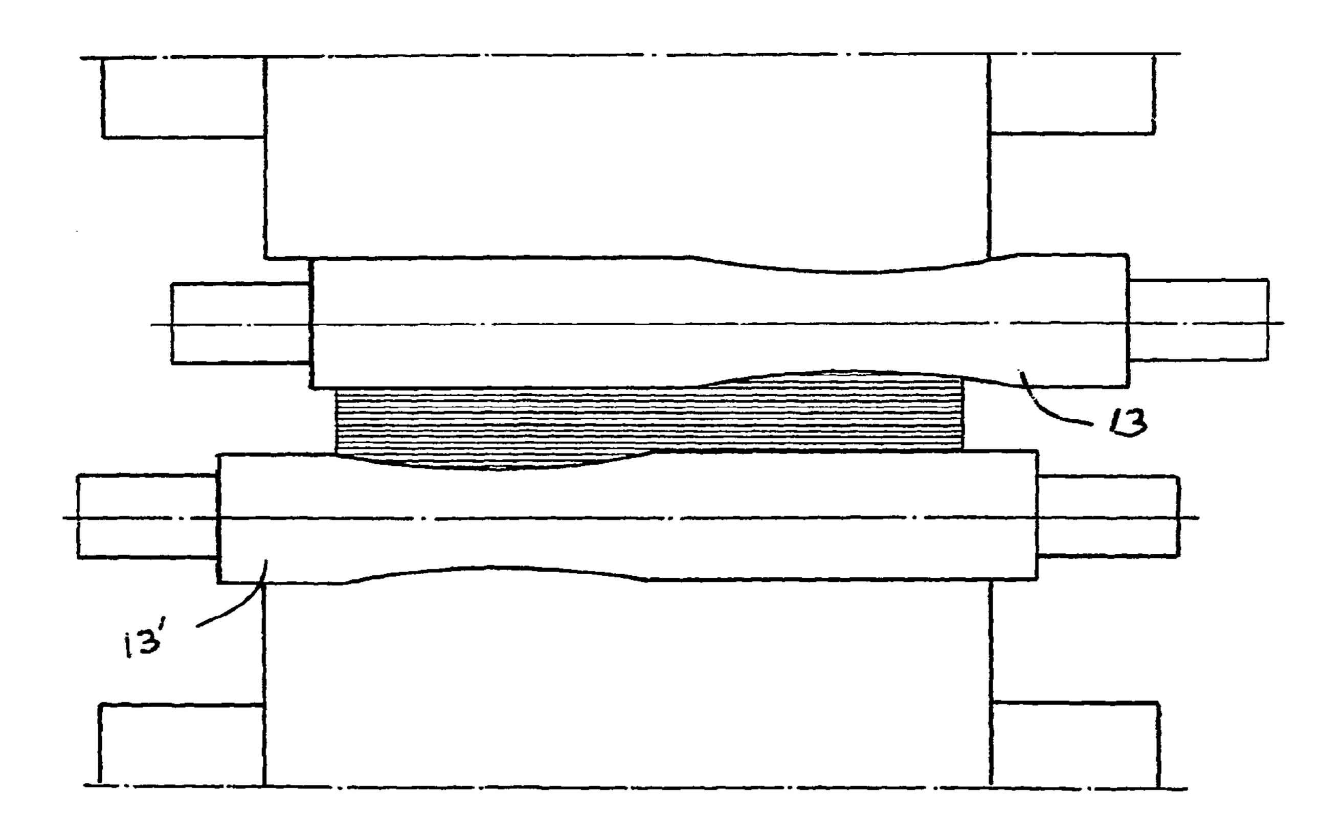
Special cross section to build up material on the strip edge
