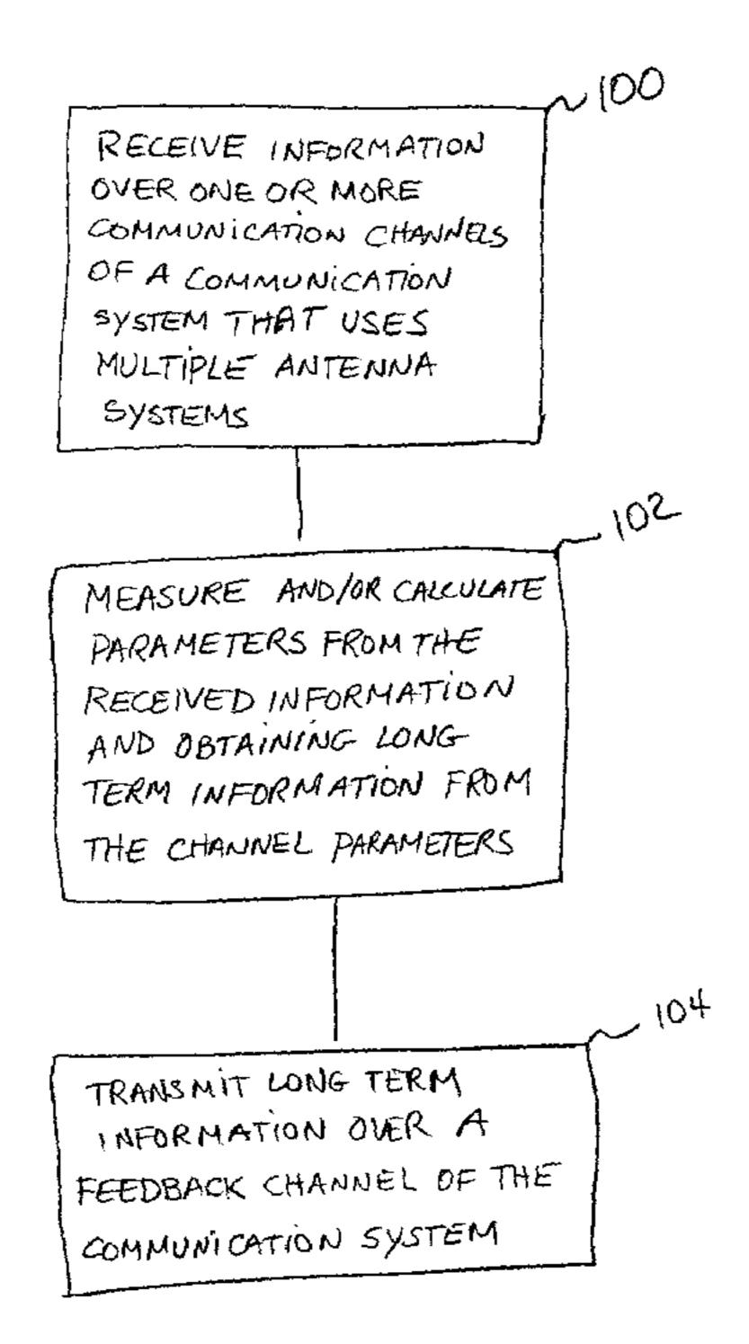
RECEIVE INFORMATION OVER ONE OR MORE COMMUNICATION CHANNELS OF A COMMUNICATION SYSTEM THAT USES MULTIPLE ANTENNA SYSTEMS
