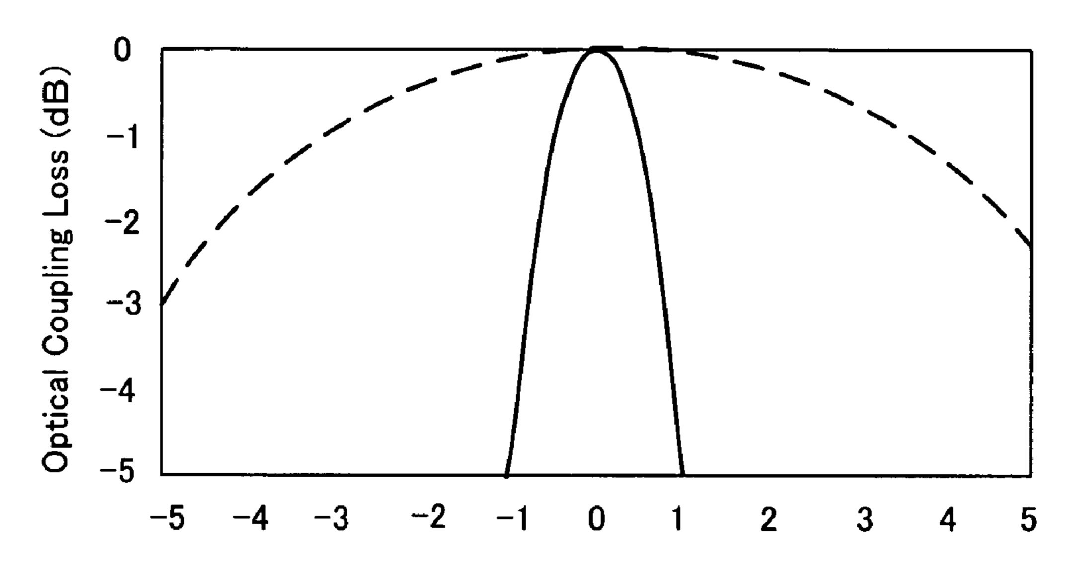
Misalingnment amount of optical axis in perpendicular direction (  $\mu$  m)
