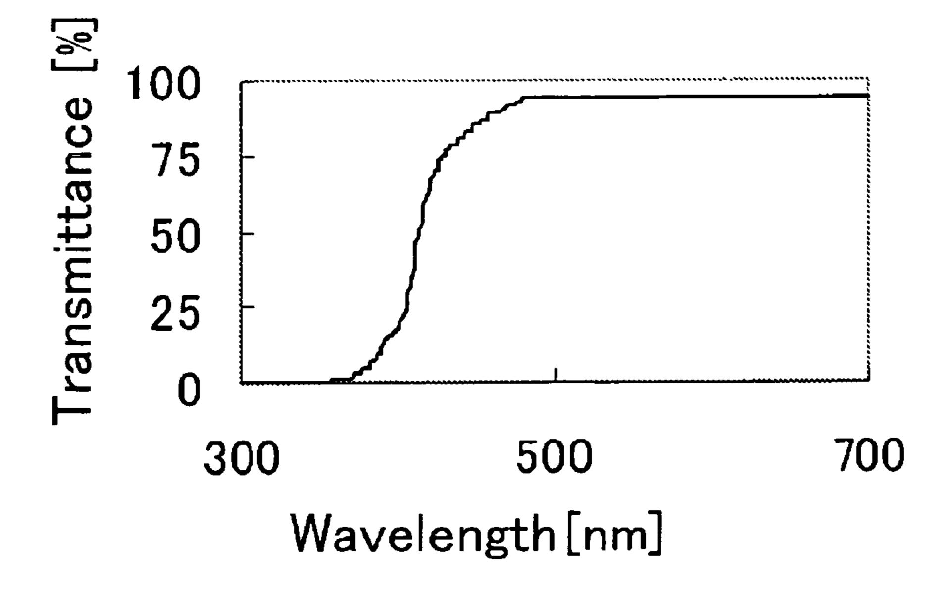
Fig.2 Transmission spectrum of the polyimide silicone in Preparation Example 5
