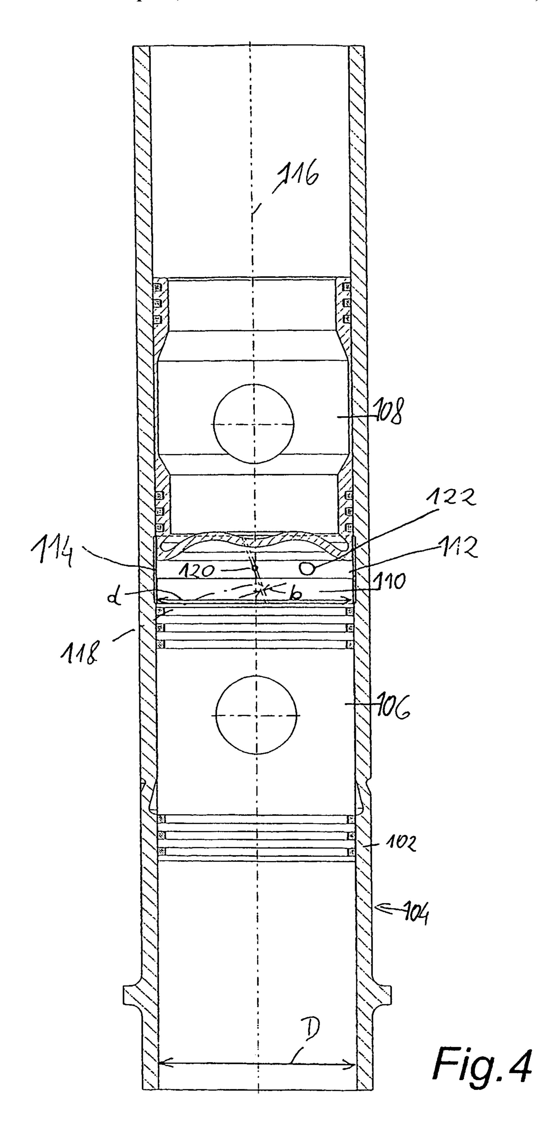
The invention relates to an internal combustion engine with at least one piston reciprocating in a cylinder, comprising a piston ring region with at least one piston ring, with the piston comprising at least a first cavity for receiving gases passing at least one compression ring, with the piston ring region of the piston being connected via at least a first manifold with the
