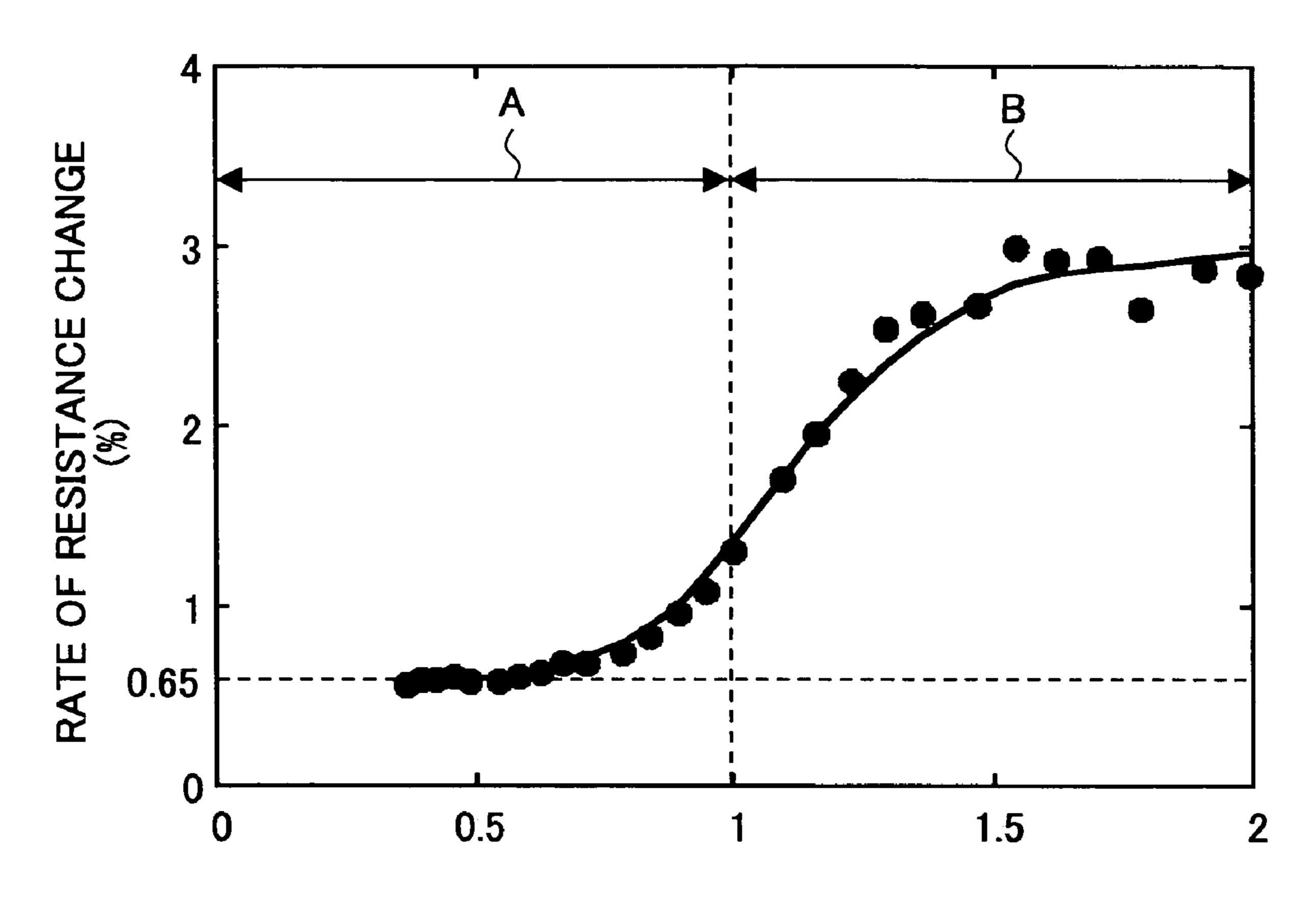
THICKNESS OF MAGNETIC INTERMEDIATE LAYER (nm)
