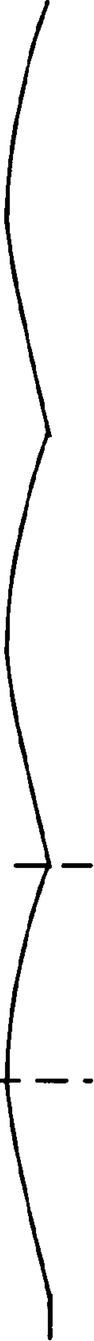
FIG. 9D OUTPUT VOLTAGE OF SMOOTHING CIRCUIT
