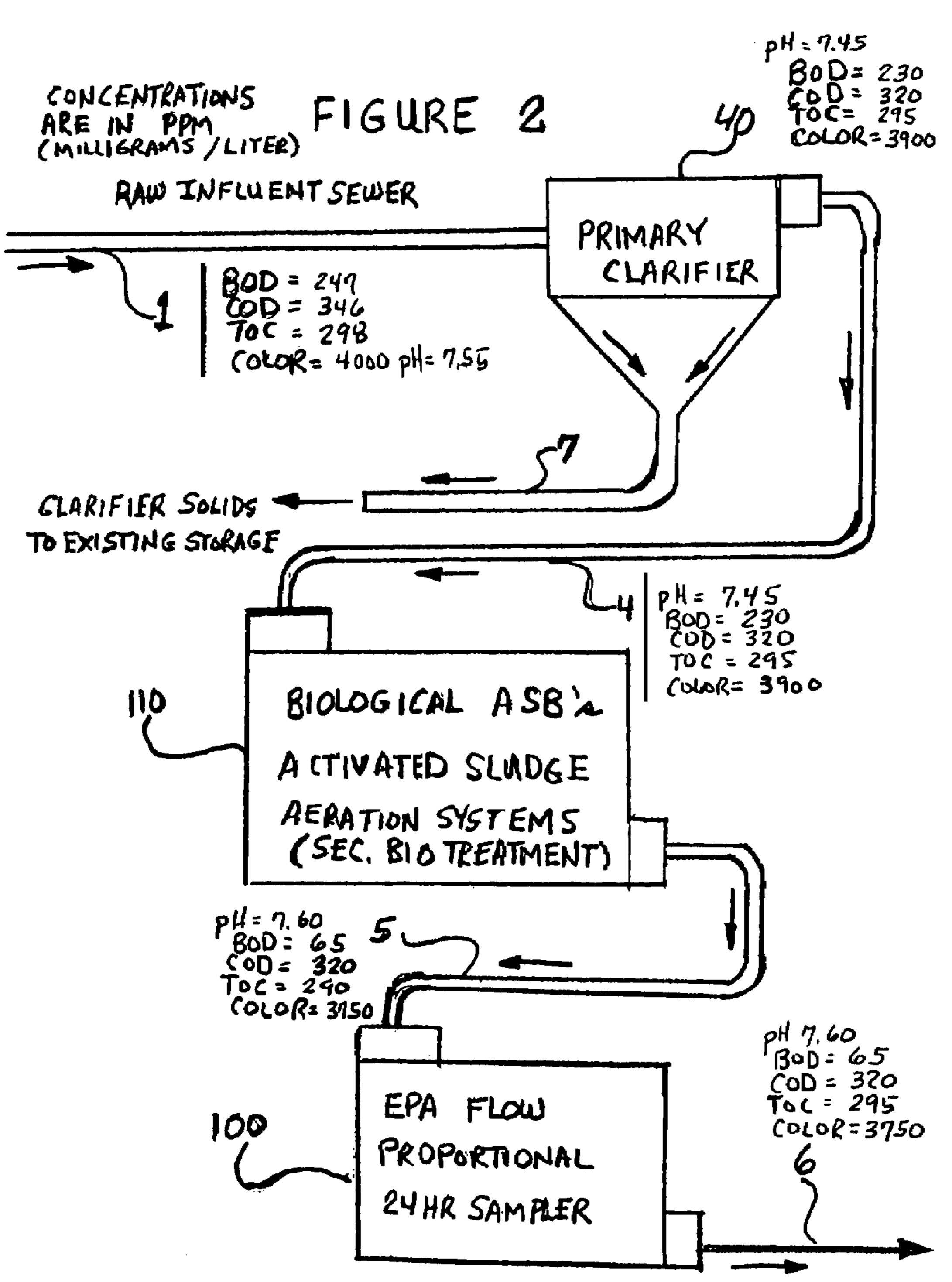
EXISTING SECONDARY BIG TREATMENT AT DERIDDER, BOISE AND IP AND BOWATER WITH NO CHEMICALS ADDED AT PRIMARY CLARIFIER
