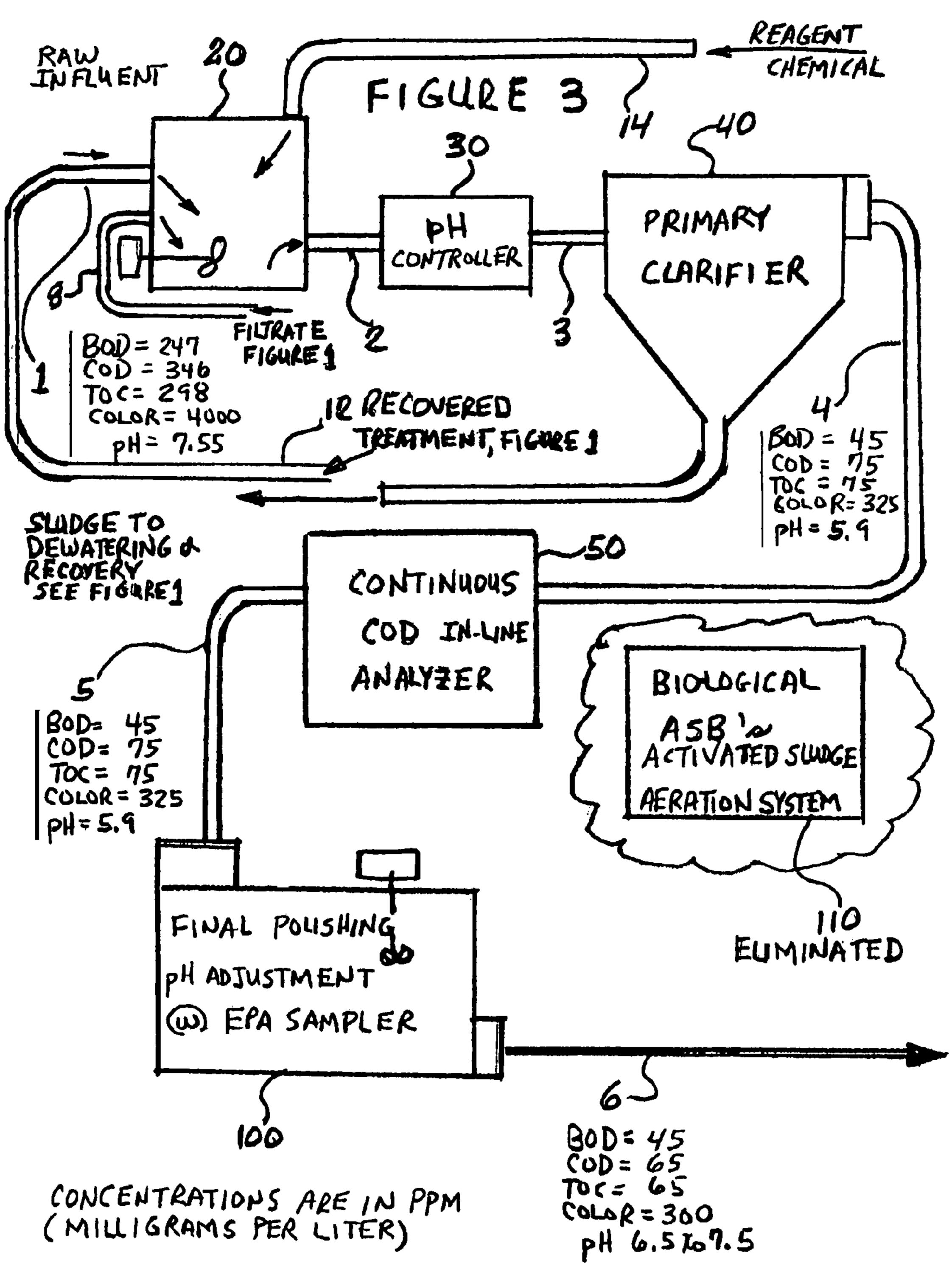
NEW INVENTION WITH CHEMICALS ADDED AT PRIMARY CLARIFIER AND BIOLOGICAL ASB'S AFRATION SECONDARY TREATMENT ELIMINATED
