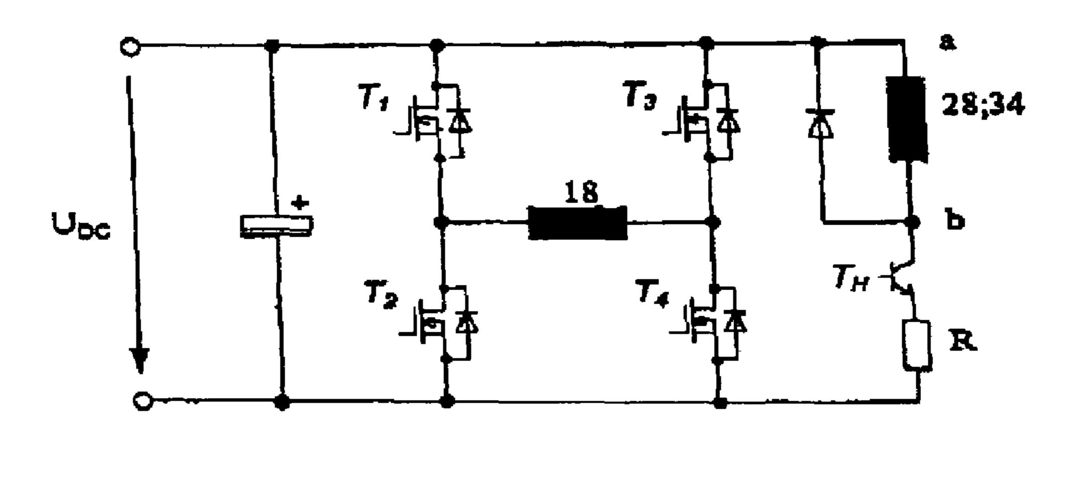
Power generator for supply the auxiliary winding
