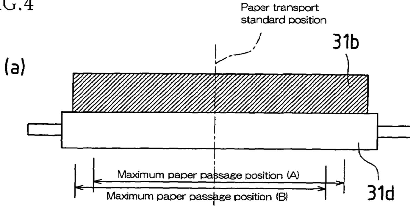
The difference between (A) and (B) changes the paper transport position of the back side using the shifter mechanism of the discharge portion used as a switchback portion.
