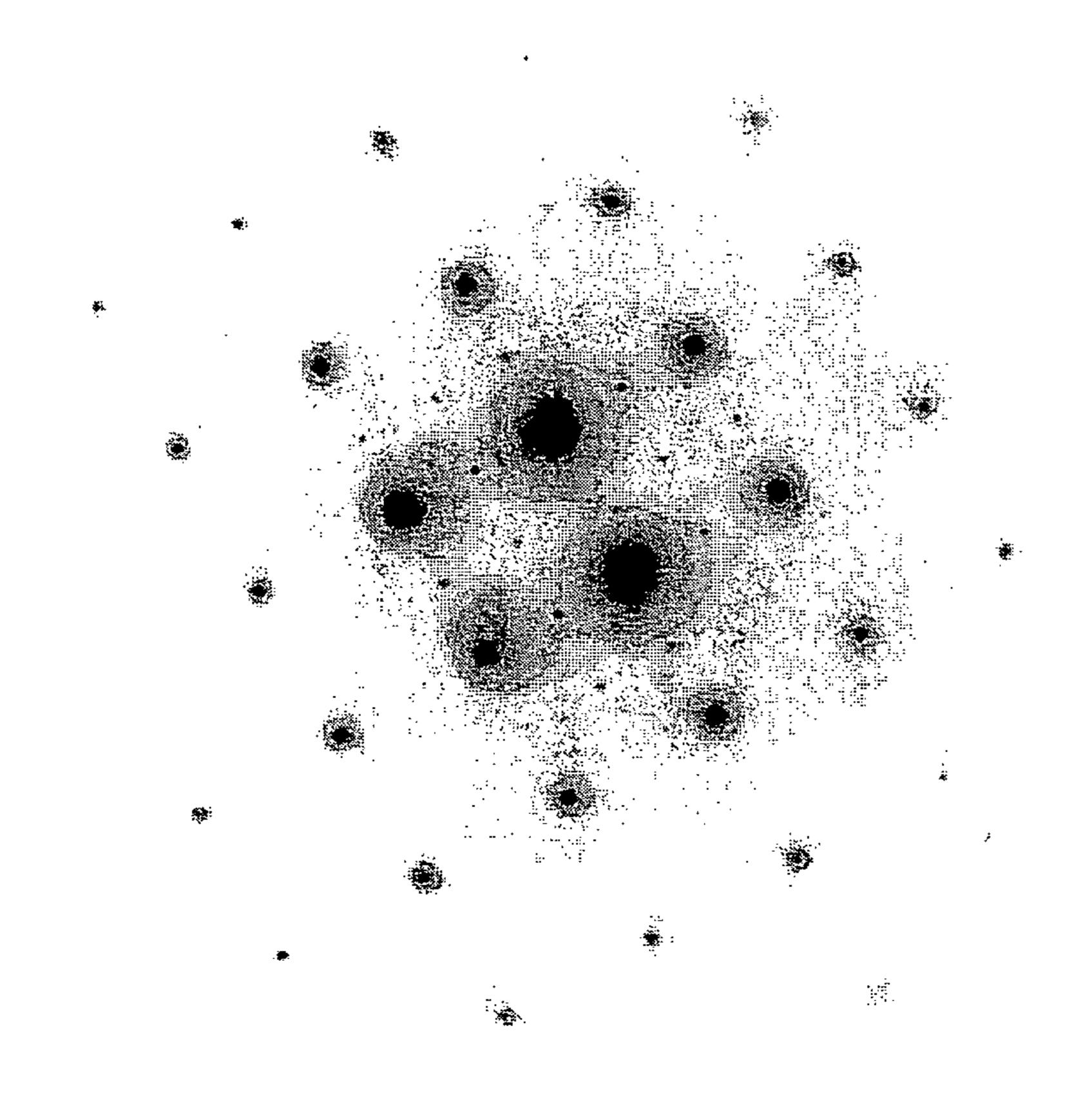
FIG. 1. Selected area diffraction pattern of Alloy #1 (heat treatment B) obtained using transmission electron microscopy (TEM) instrument, showing matrix and  $\gamma'$  diffracted spots.
