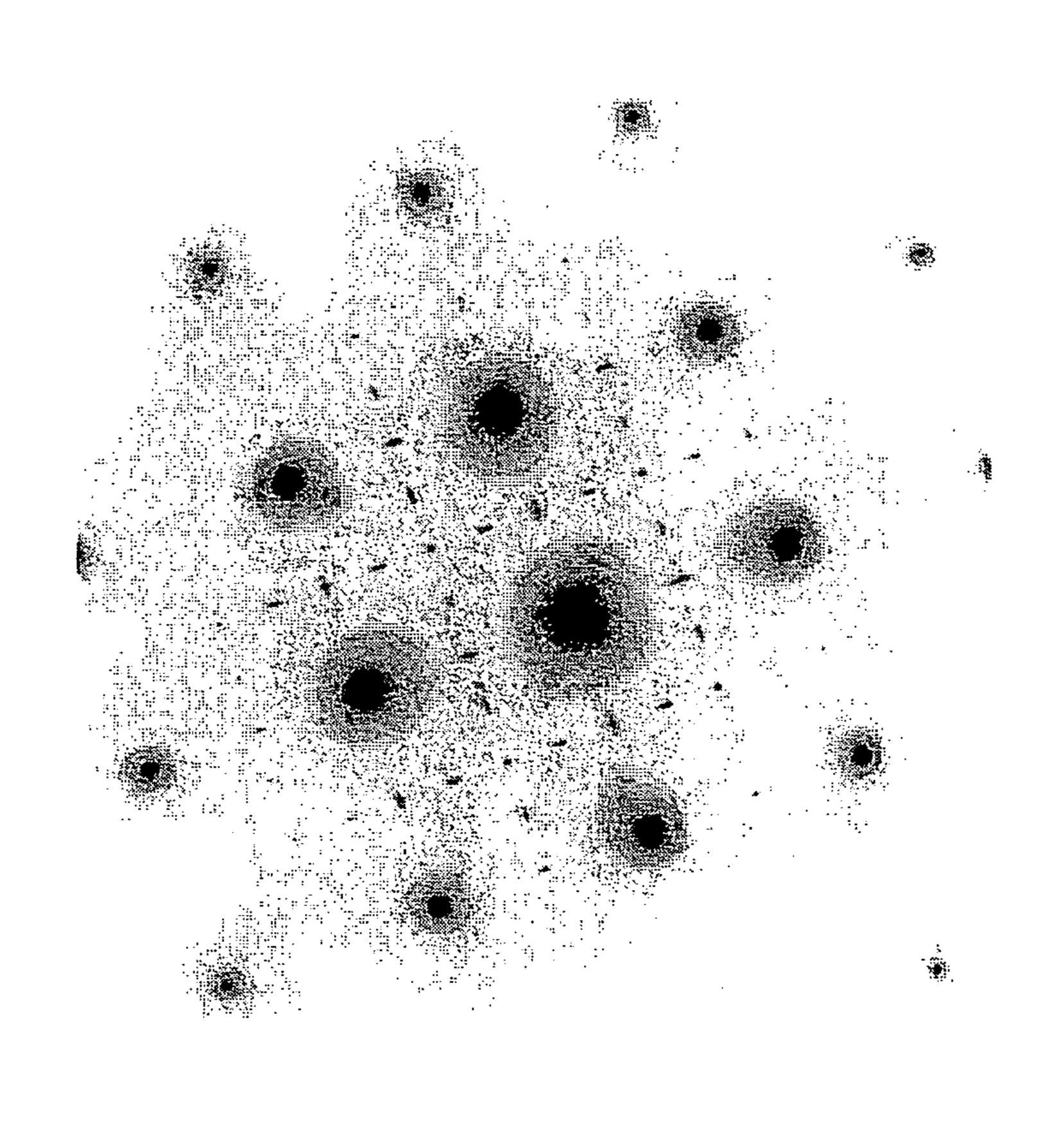
FIG. 2. Selected area diffraction pattern of Alloy #7 (heat treatment C) obtained using transmission electron microscopy (TEM) instrument, showing matrix,  $\gamma'$  and  $\gamma''$  diffracted spots. The streaks are generated by the presence of  $\gamma''$ .
