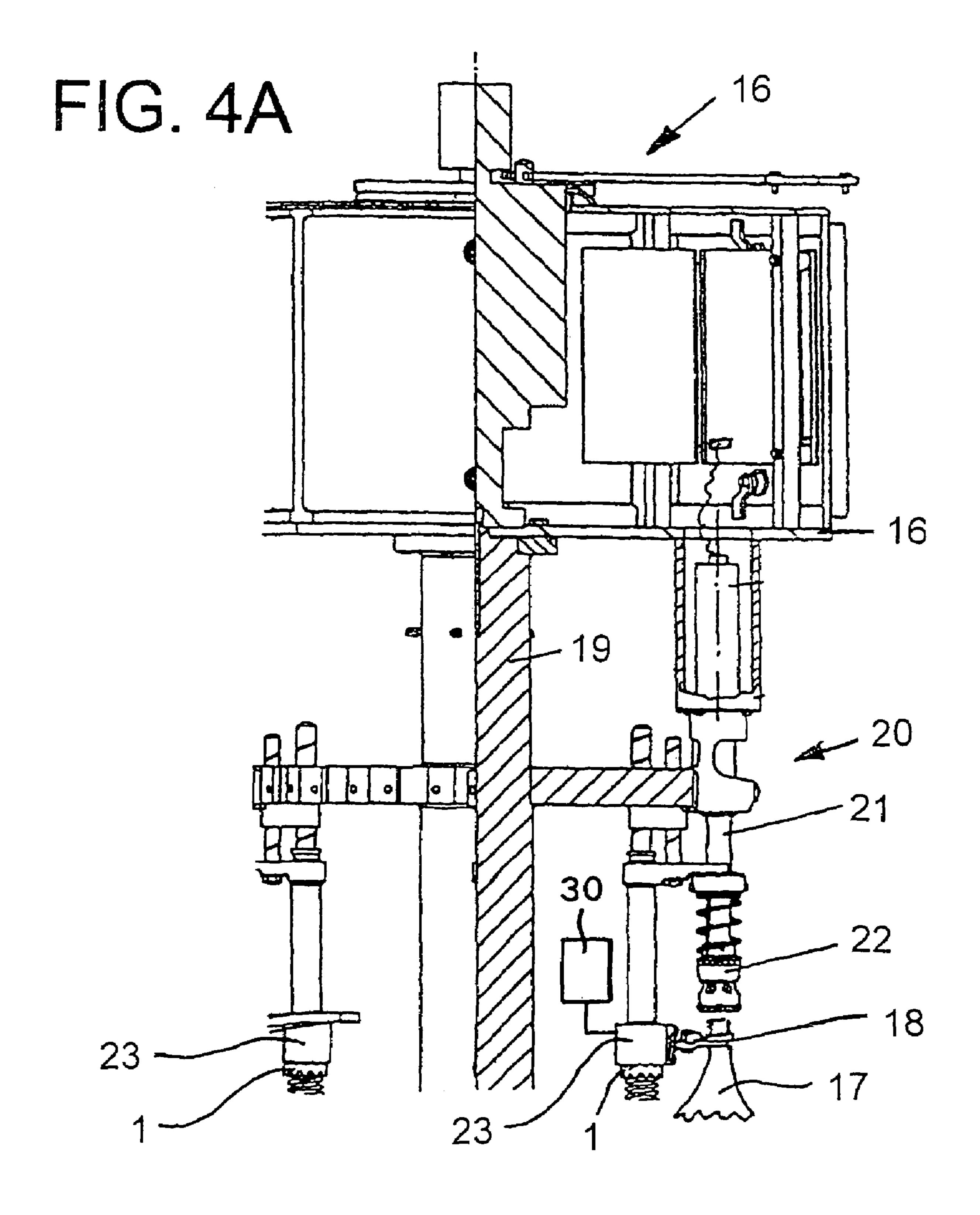
BEVERAGE BOTTLING PLANT HAVING A BEVERAGE BOTTLE CLOSING MACHINE WITH A BEARING SYSTEM TO GUIDE A RECIPROCATING SHAFT IN THE BEVERAGE BOTTLE CLOSING MACHINE
