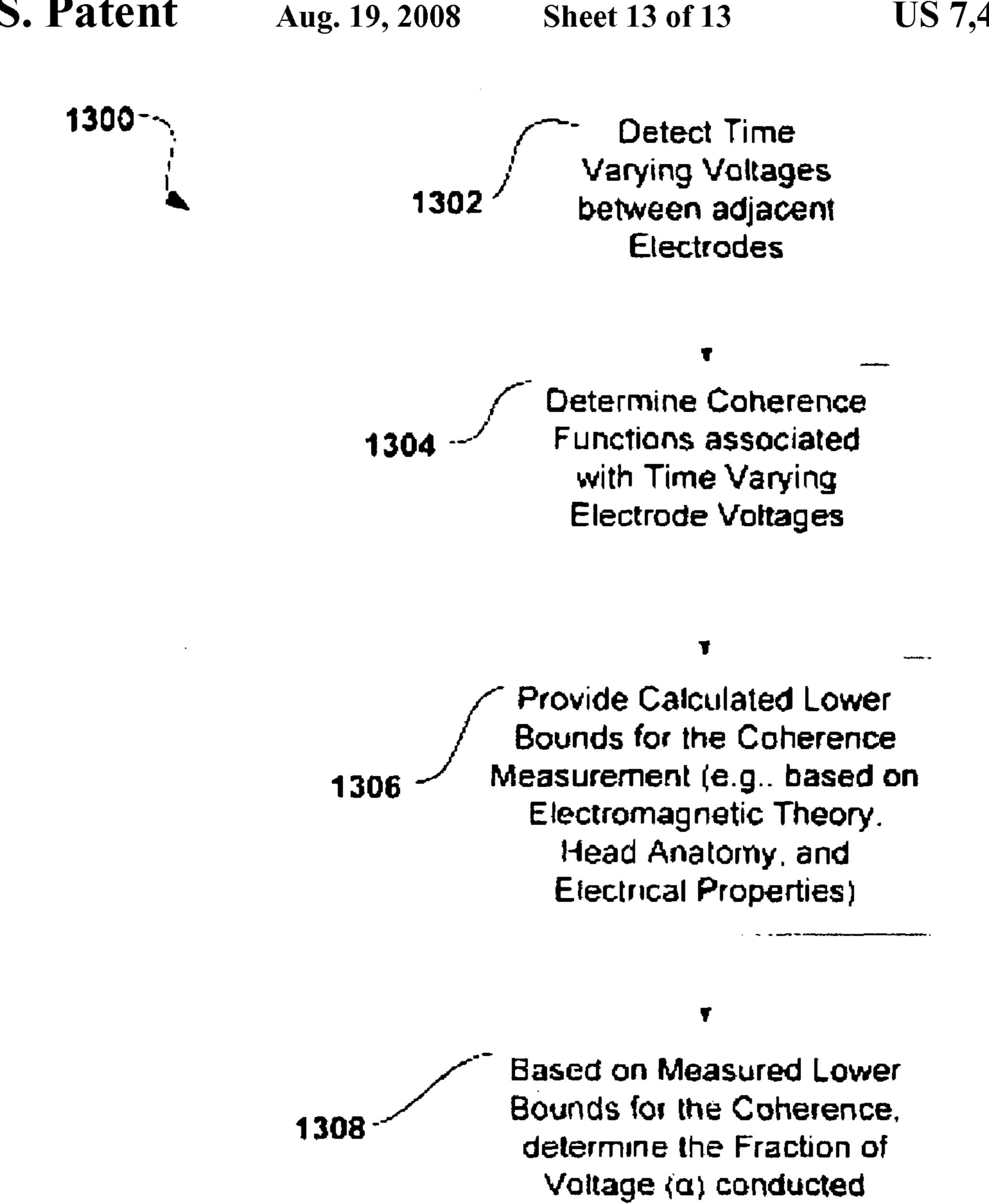
Based on Calculated Lower Bounds for the Coherence Measurement and the determined Fraction of Voltage (a). Calculate the error-compensated Coherence between electrode signals by solving the Coherence equations.
