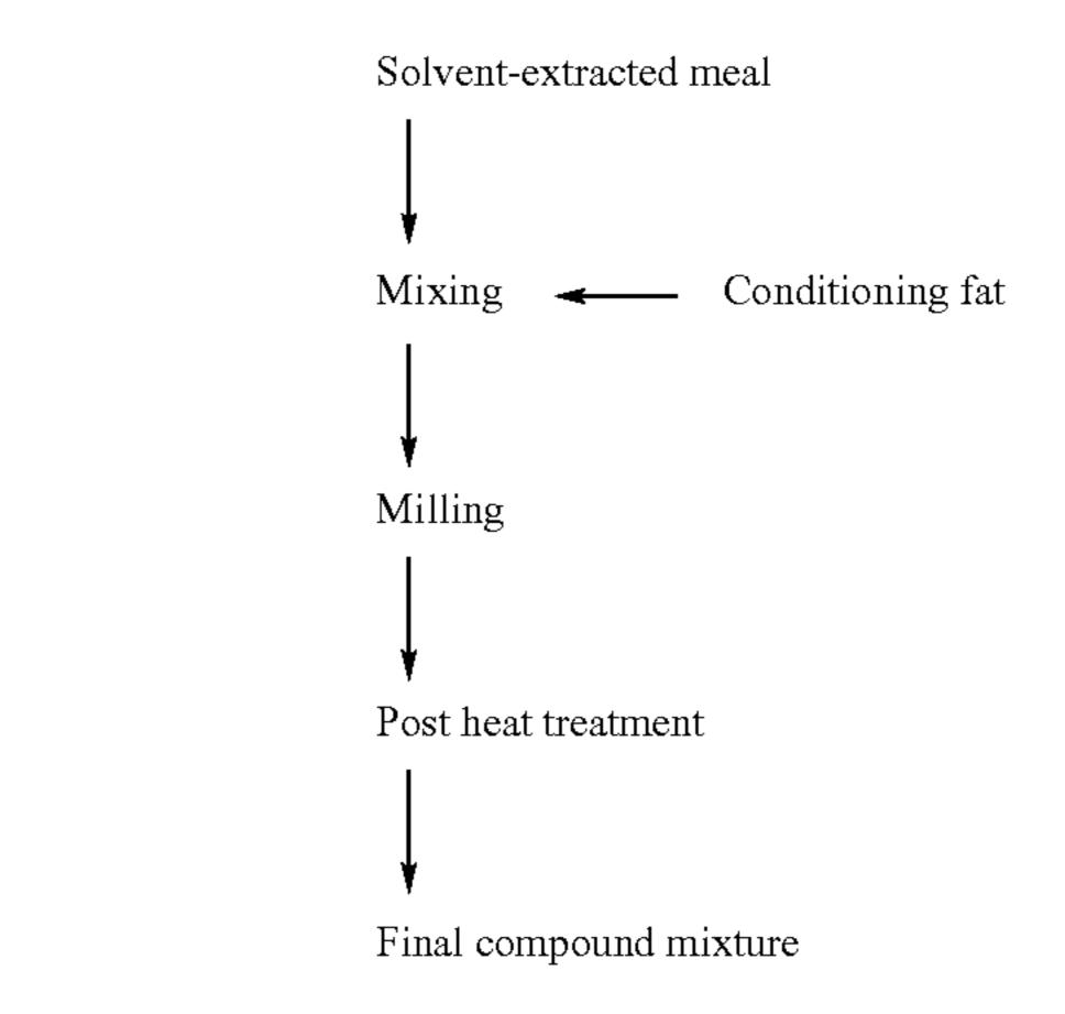
Apparatus for Treating Solvent-Extracted Plant R sidu
