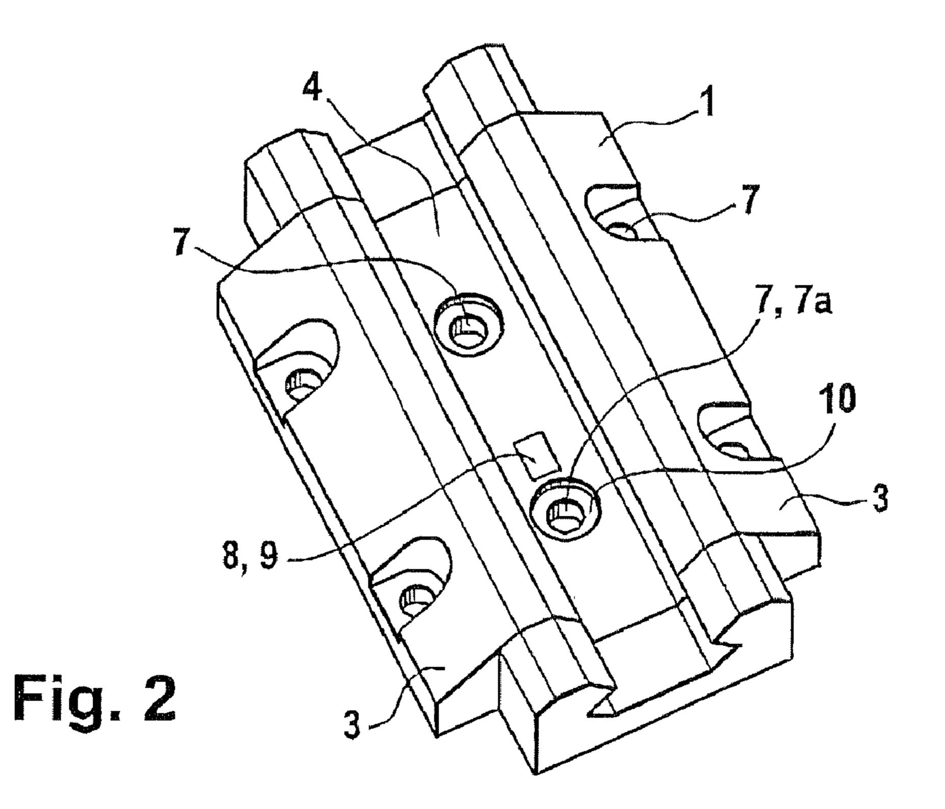
The present invention relates to a linear rolling bearing having an approximately U-shaped guide carriage which is arranged in a longitudinally displaceable manner on a guide rail.
