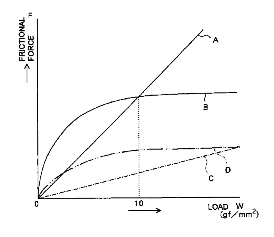
A: FRICTIONAL FORCE BETWEEN SURFACE OF THERMAL HEAD AND HEAT-SENSITIVE ADHESIVE LAYER (NON-ACTIVATED PORTION)
