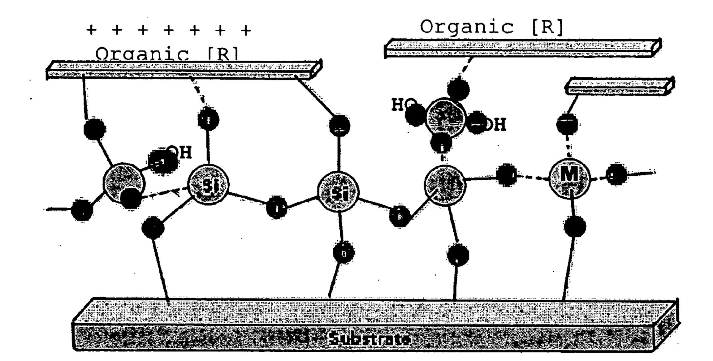
This simplified model of cured siloxane applied as a reactive silanol illustrating organic groups oriented at the surface of an interpenetrating network of siloxane covalently bonded to the substrate.
