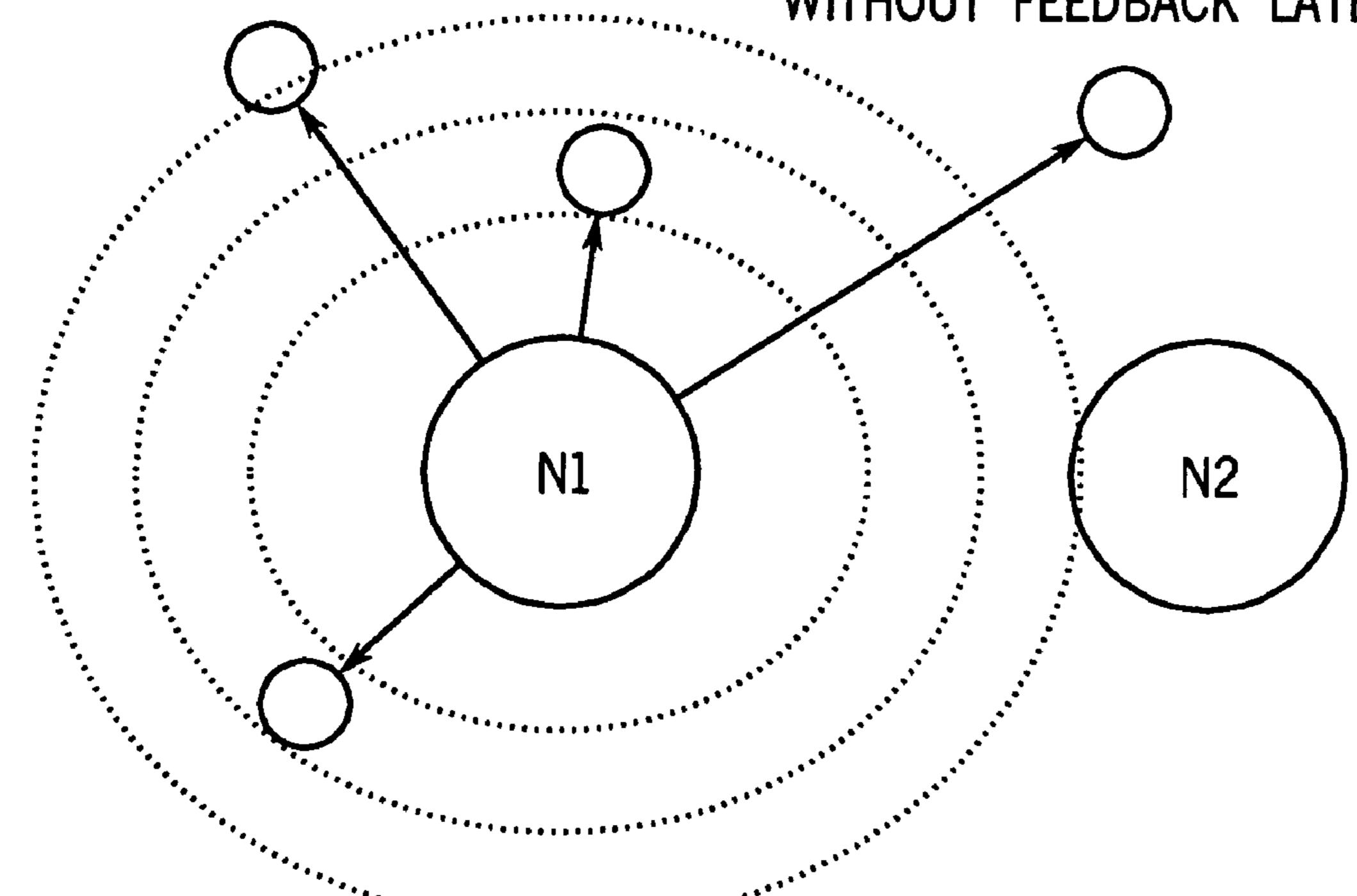
N1 INCLUDES TX POWER IN ALL TRANSMISSION HEADERS FOR METRIC NORMALIZATION AT N2
