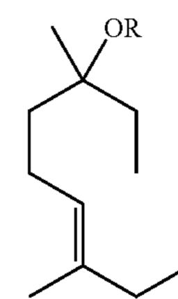
wherein R represents a hydrogen or a straight, branched or cyclic hydrocarbon moiety consisting of less than 15, preferably less than 10, most preferably less than 4 carbon atoms and containing at least one oxygen atom and a single and/or double bonds.
