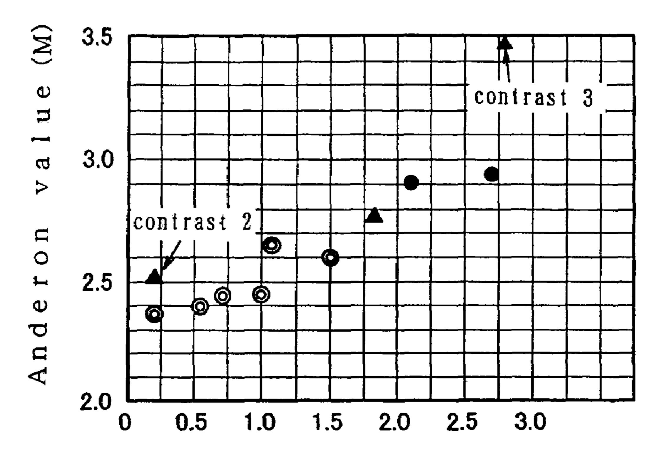
Average value of circle equivalent diameters of eutectic carbides ( $\mu m$ )
