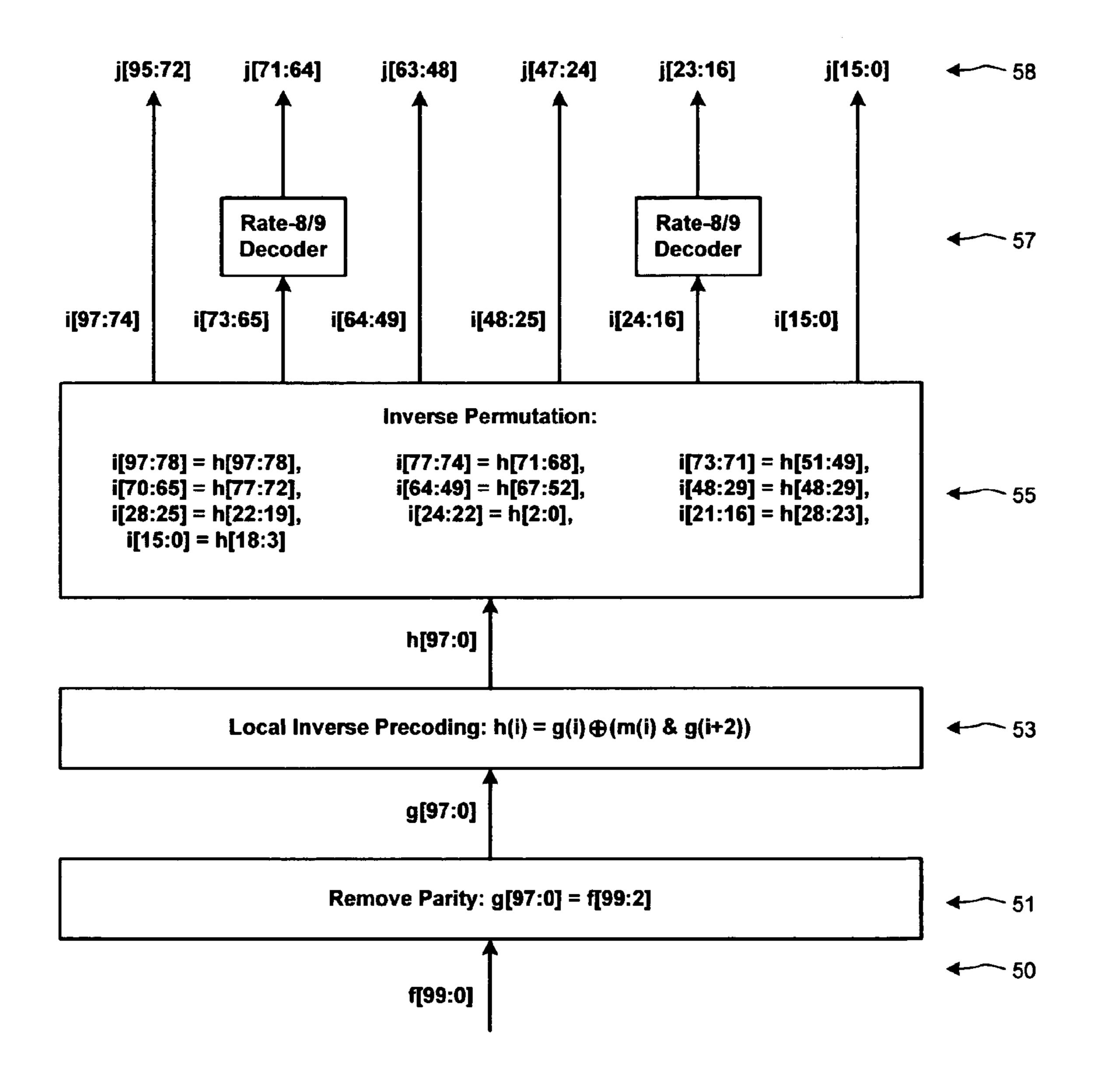
Rate-96/100 decoder for 8-bit ECC (2 parity bits)
