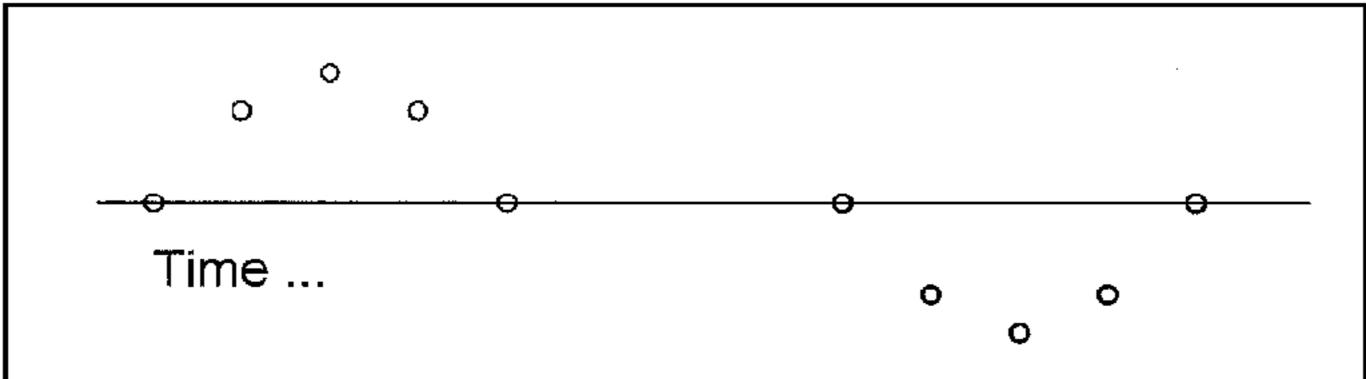
Figure 6. Digitization of an echo having separated hill and valley
