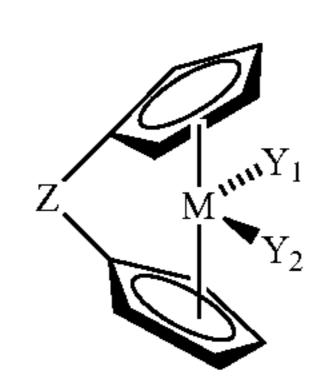
wherein  $Y_1$  and  $Y_2$ = $C_1$ - $C_{20}$  hydrocarbyl or silahydrocarbyl radicals or halogen; M=Ti, Zr, or Hf; Z=a  $C_1$ - $C_6$  hydrocarbyl, silahydrocarbyl, or silyl bridge radical; and the cyclopentadienyls may be substituted with hydrogen, halogens, or  $C_1$ - $C_{20}$  hydrocarbon or silahydrocarbyl radicals and may be multi-ring including substituted indenyl.
