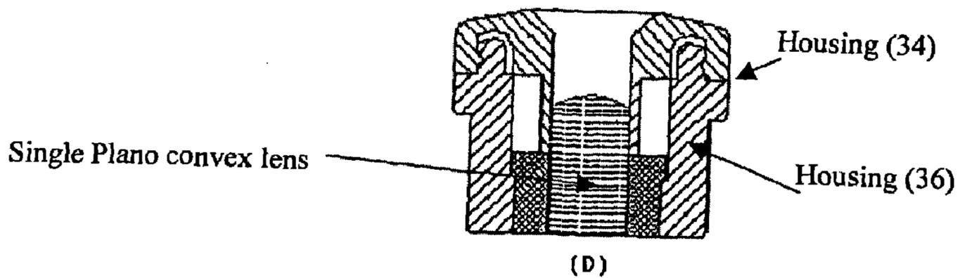
**FIGURE 5: FIXED FOCUS EYEPIECE ASSEMBLY**
