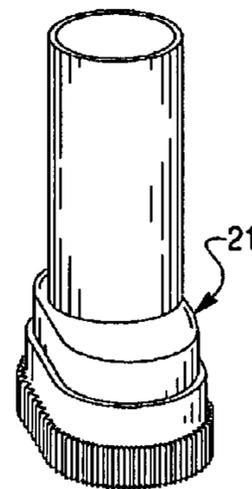
FIGURE 4: FIXED FOCUS EYEPIECE ASSEMBLY
