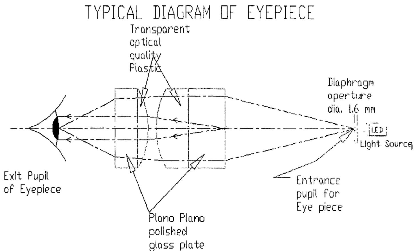
**FIGURE 9: COMPLETE OPTICAL RAY PATH INSIDE THE EYEPiece HAVING BI-CONVEX LENS**
