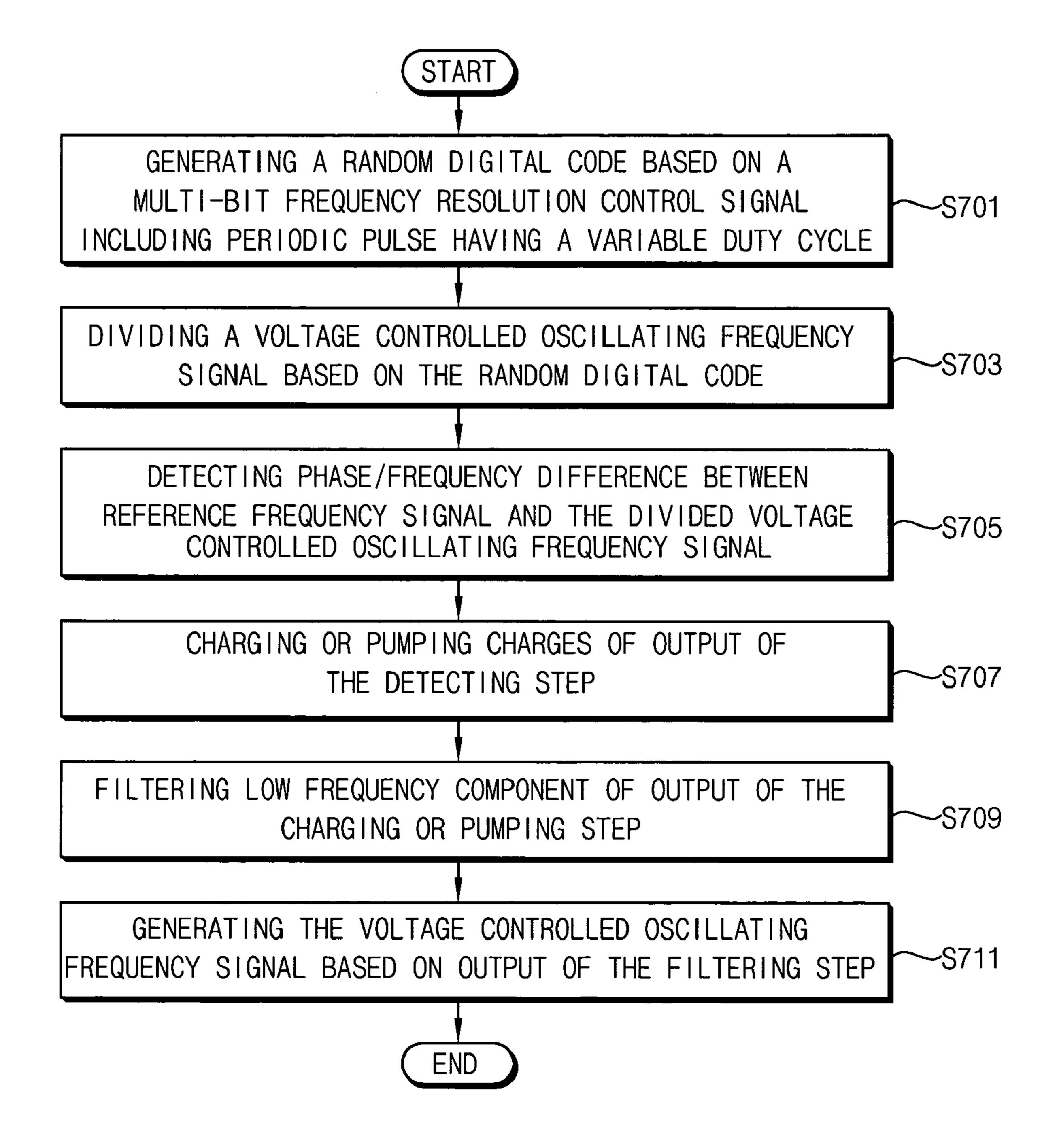
FREQUENCY SYNTHESIZER HAVING VARIABLE FREQUENCY RESOLUTION, AND FRACTIONAL-N FREQUENCY SYNTHESIZING METHOD USING SIGMA-DELTA MODULATION OF FREQUENCY CONTROL PULSES
