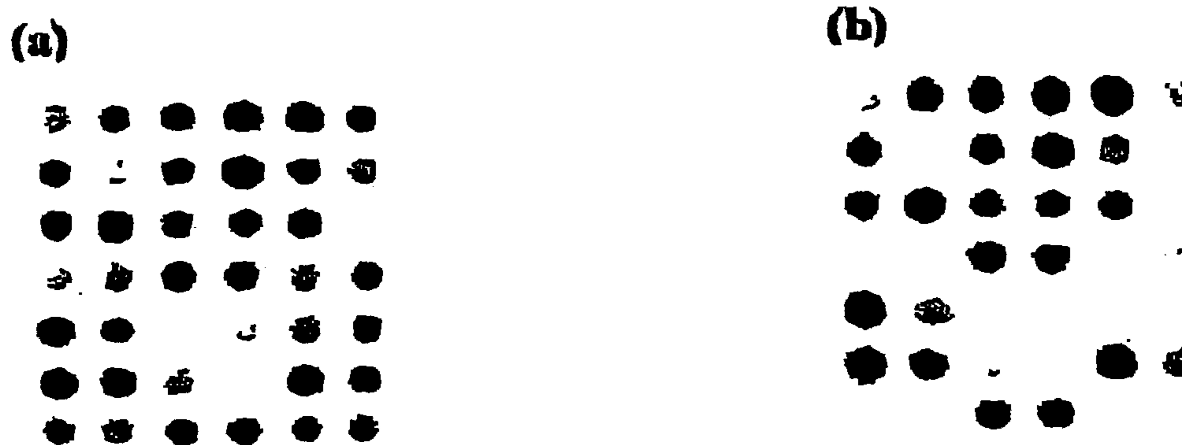
Figure 5. The assay images of spots printed with the spotting solution containing 0.0018% (w/v) of N-Isocetyl sarcosine (NIS) in 45 mM borate buffer at pH 9.3. After printing, the microarrays were incubated at room temperature with a) 70% RH (relative humidity) or b) 95% RH.
