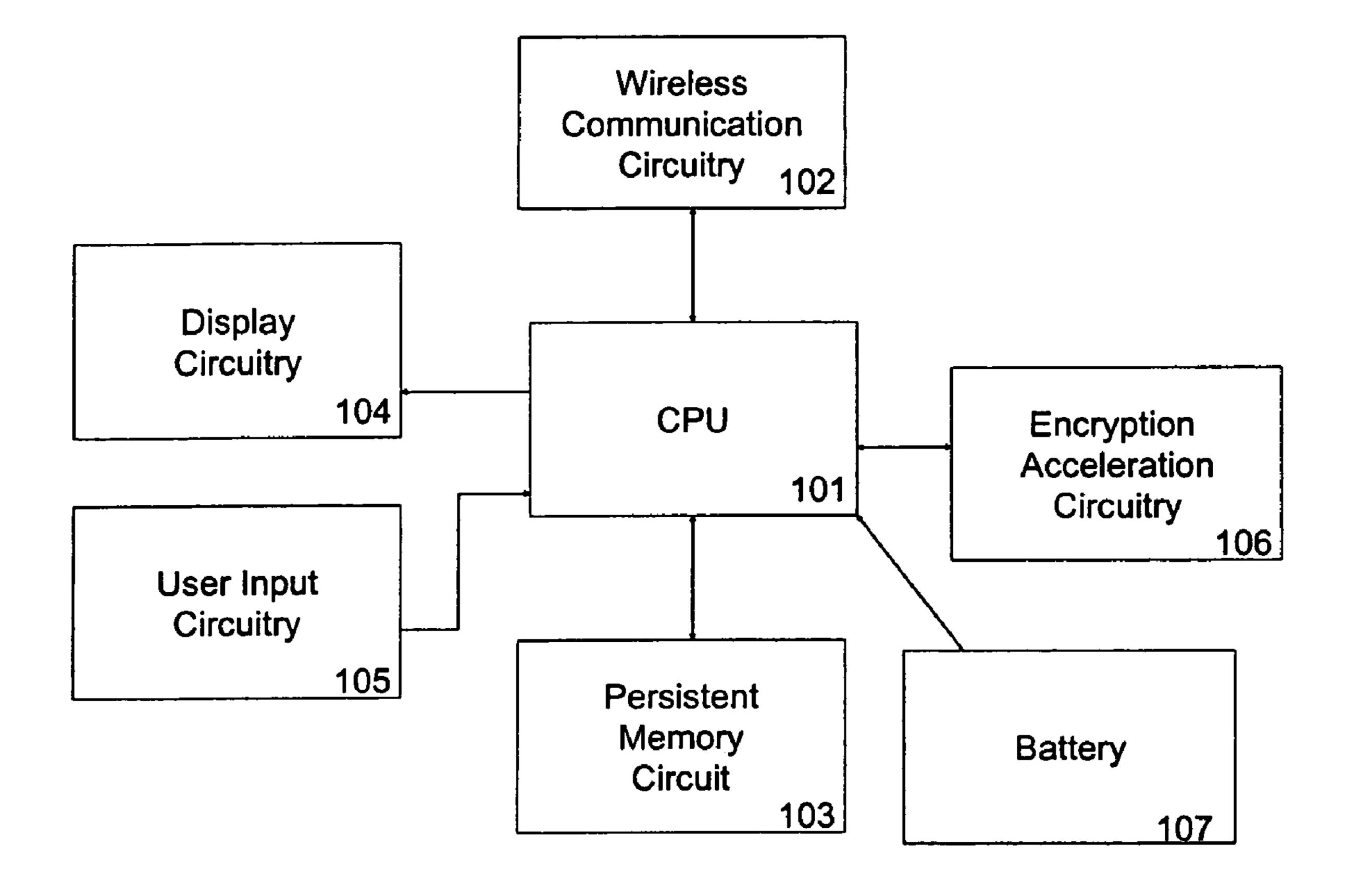
Fig. 1 Block Diagram of Universal ID Card
