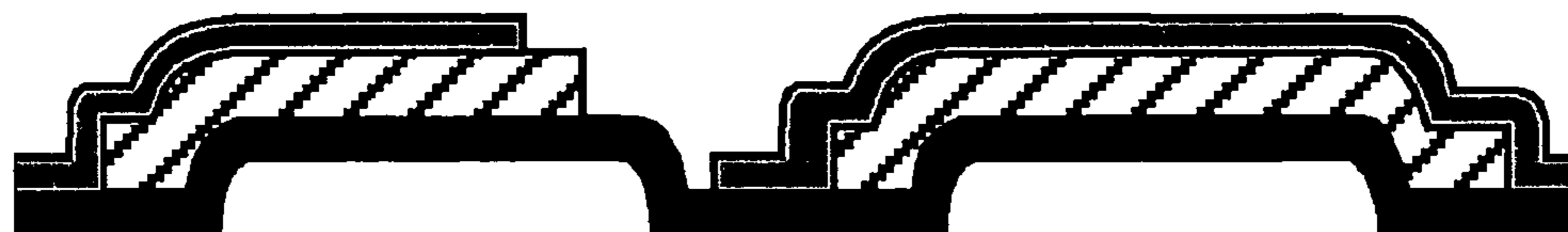
Before the release of a mechanical structure via the removal of the sacrificial layer
