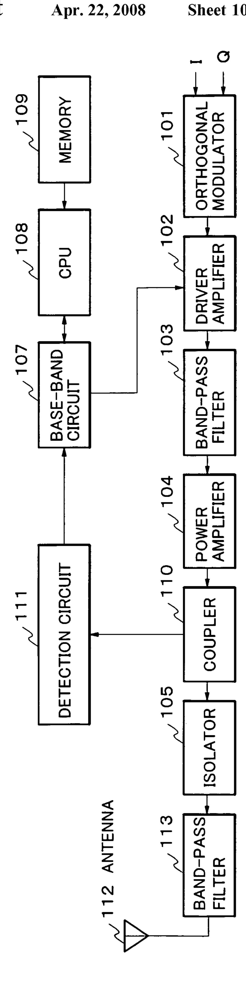
TRANSMISSION POWER CONTROL DEVICE AND METHOD THEREOF, COMPUTER PROGRAM FOR TRANSMISSION POWER CONTROL DEVICE, AND RADIO TRANSMITTER
