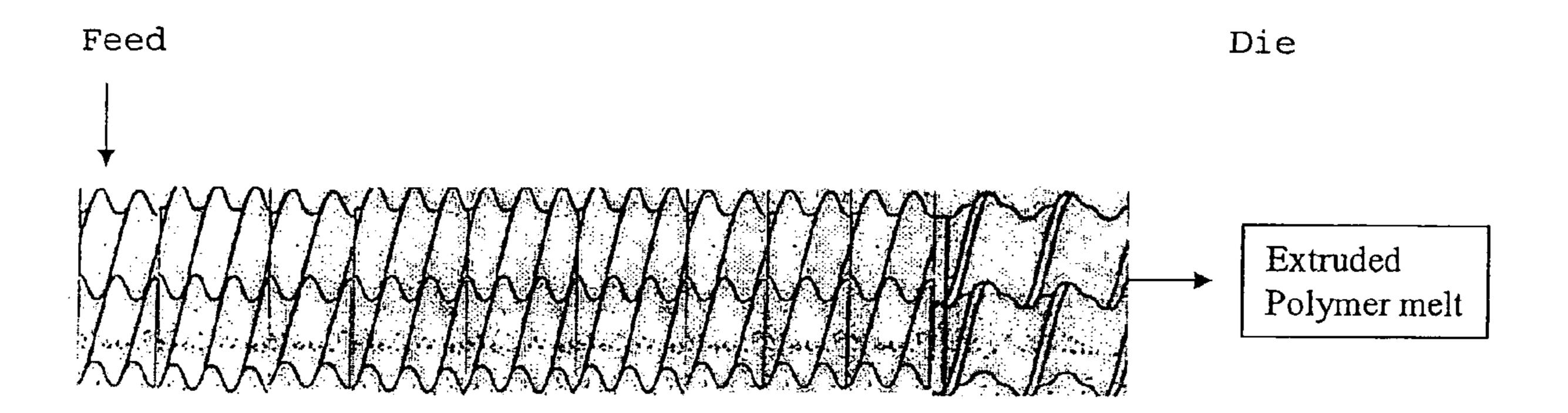
Figure 1: Screw configuration
