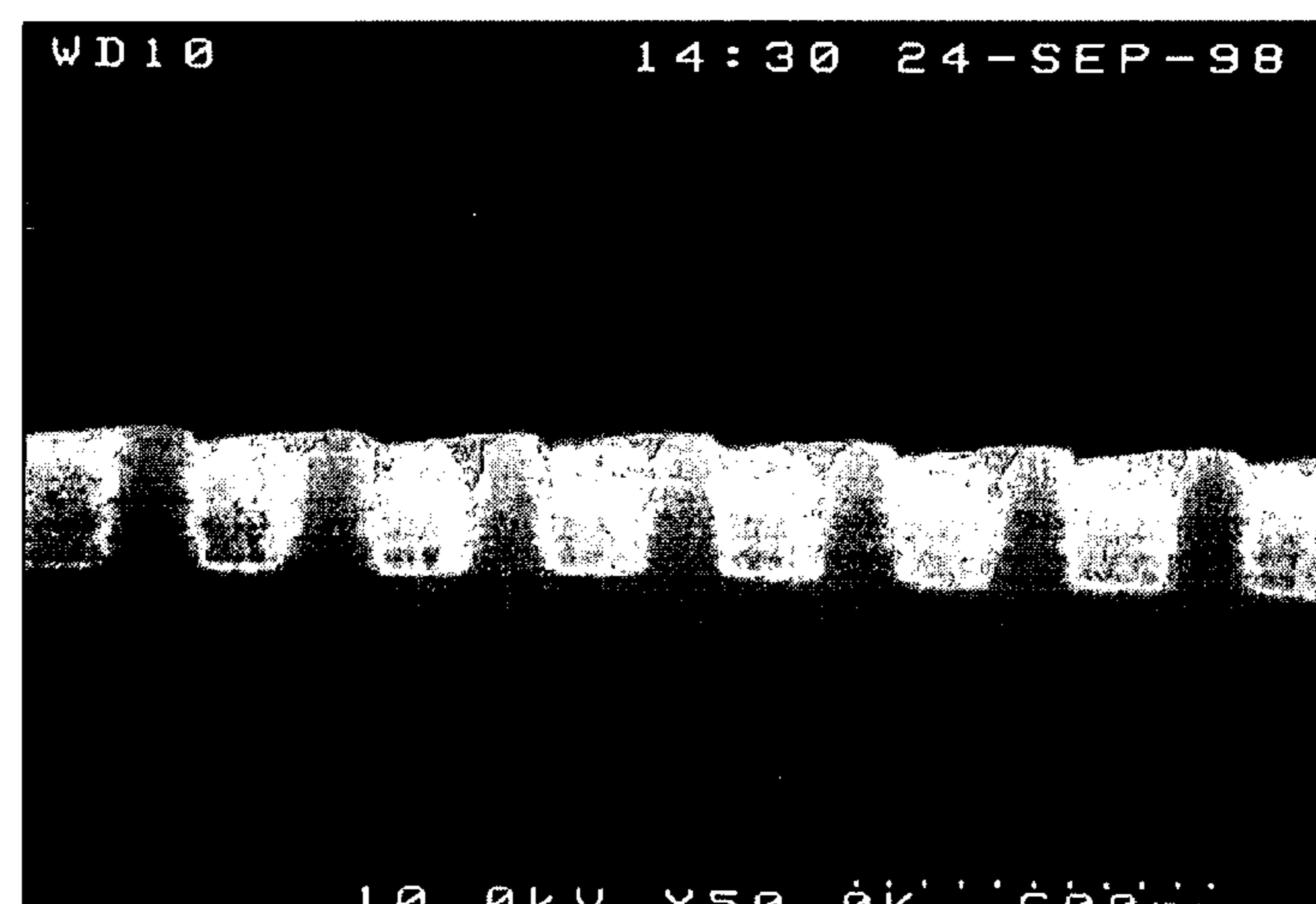
novolak underlayer with k=0.08 at 248nm
