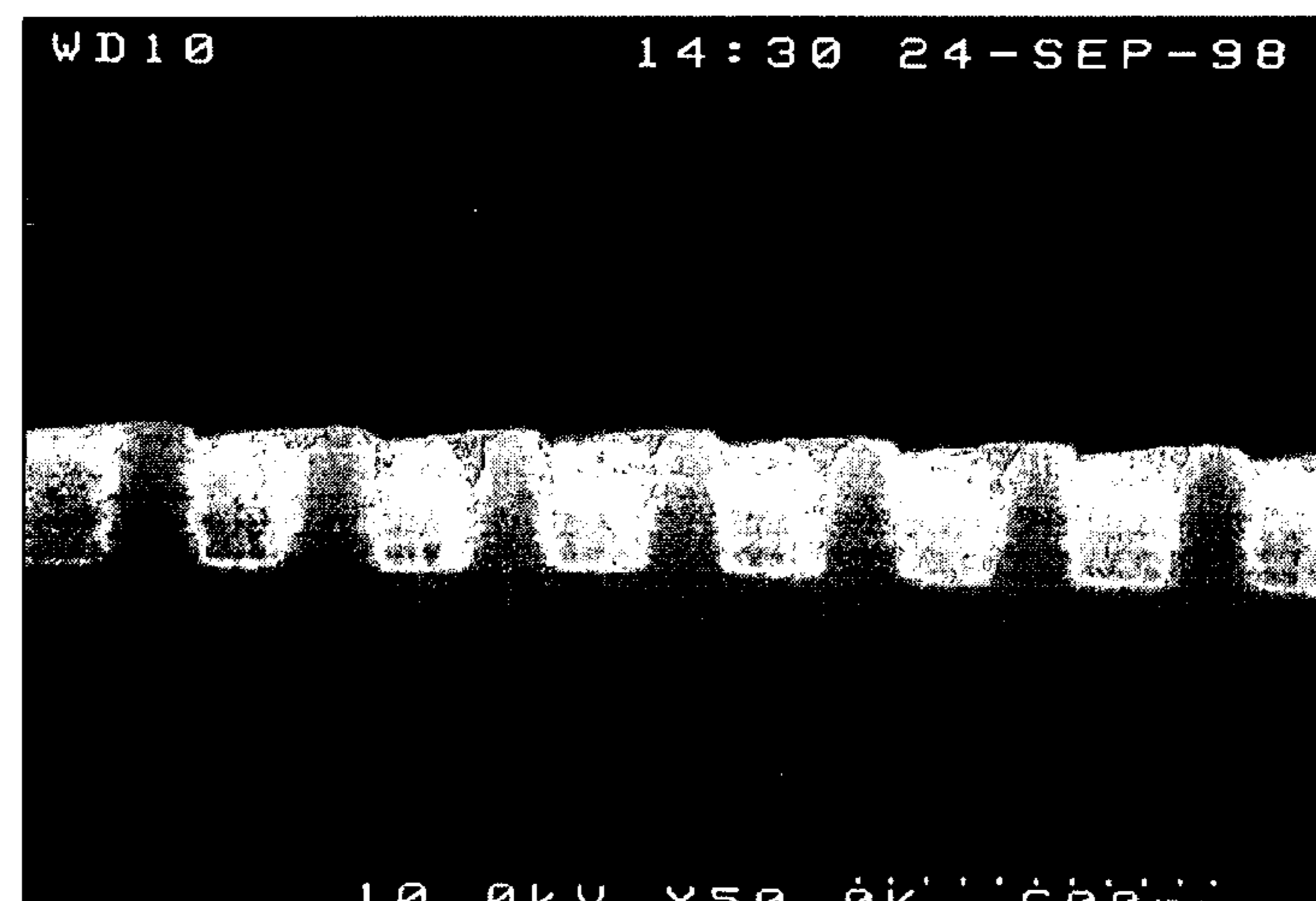
novolak underlayer with k=0.08 at 248nm
