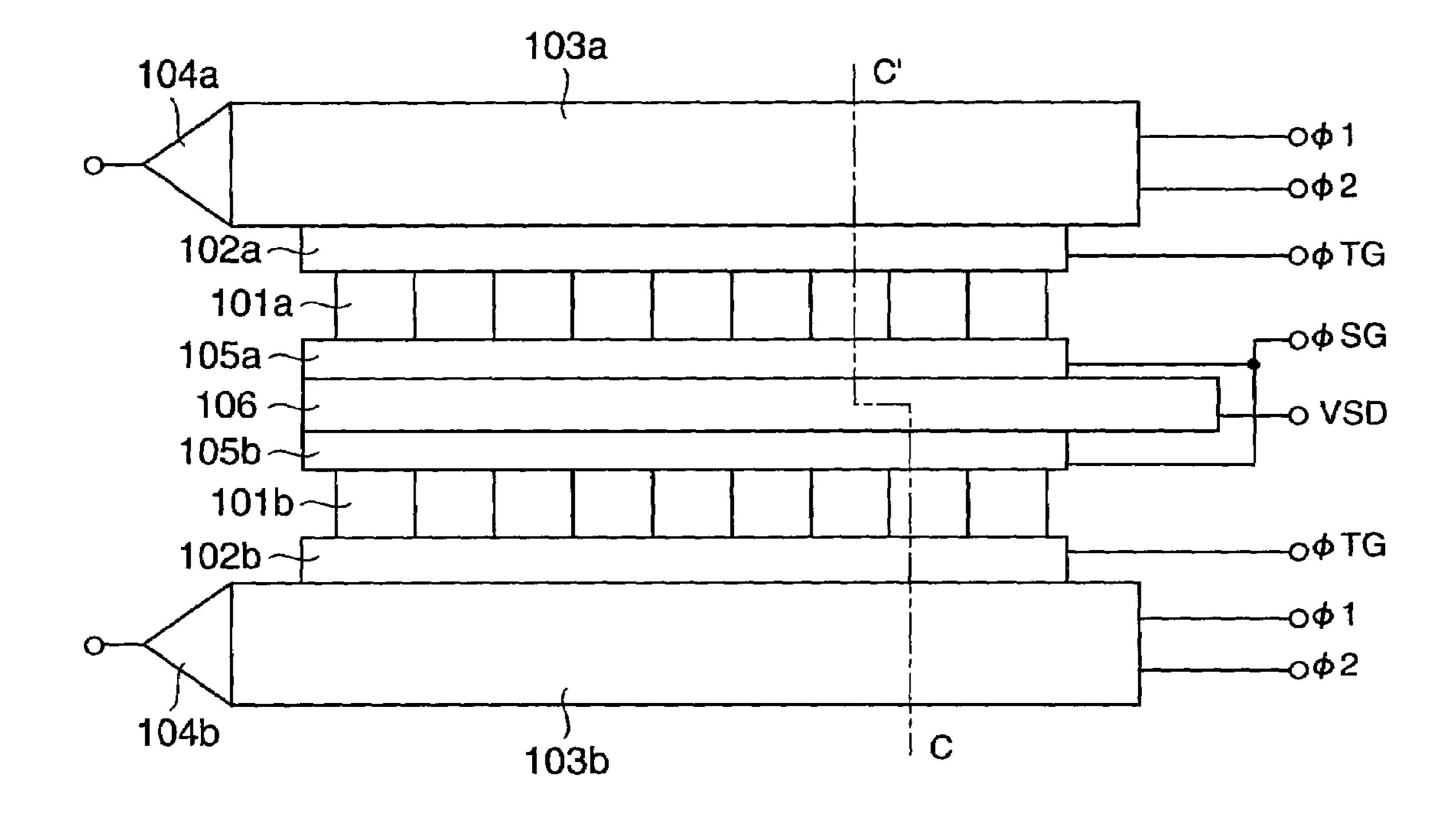
101a,101b PHOTODIODE ARRAY 103a,103b CCD SHIFT REGISTER 105a,105b SHUTTER GATE
