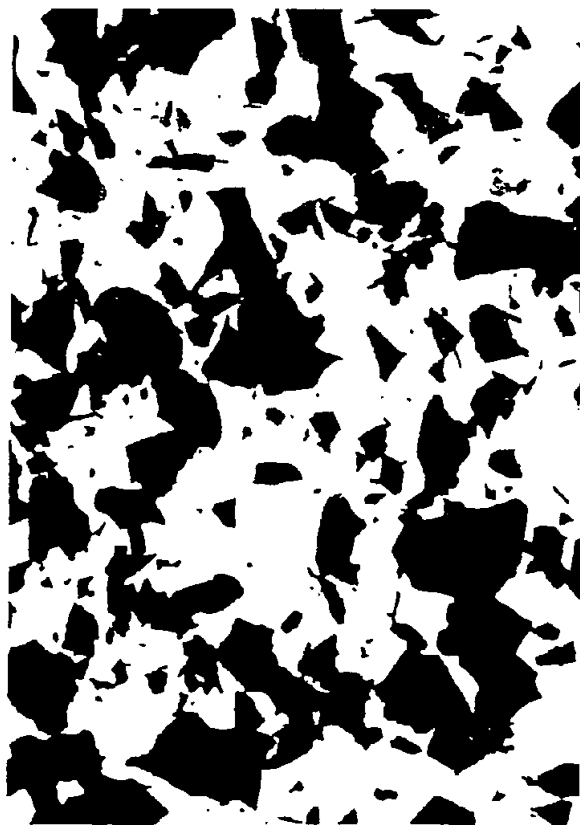
Fig. 1 Optical micrograph of MIOX SG
