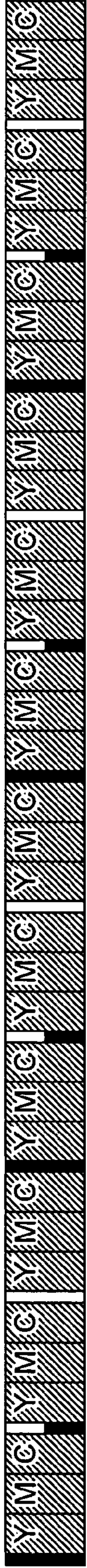
FIG. 5(A) Mark A with cycle period comprising 3 unit frames (a12)
