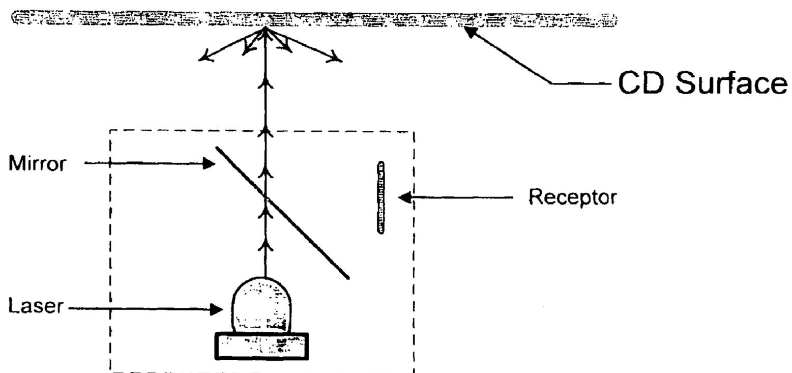
In this diagram, the laser light strikes a pit on the CD surface and is scattered. No light is reflected to the receptor and the output is a binary '0'.
