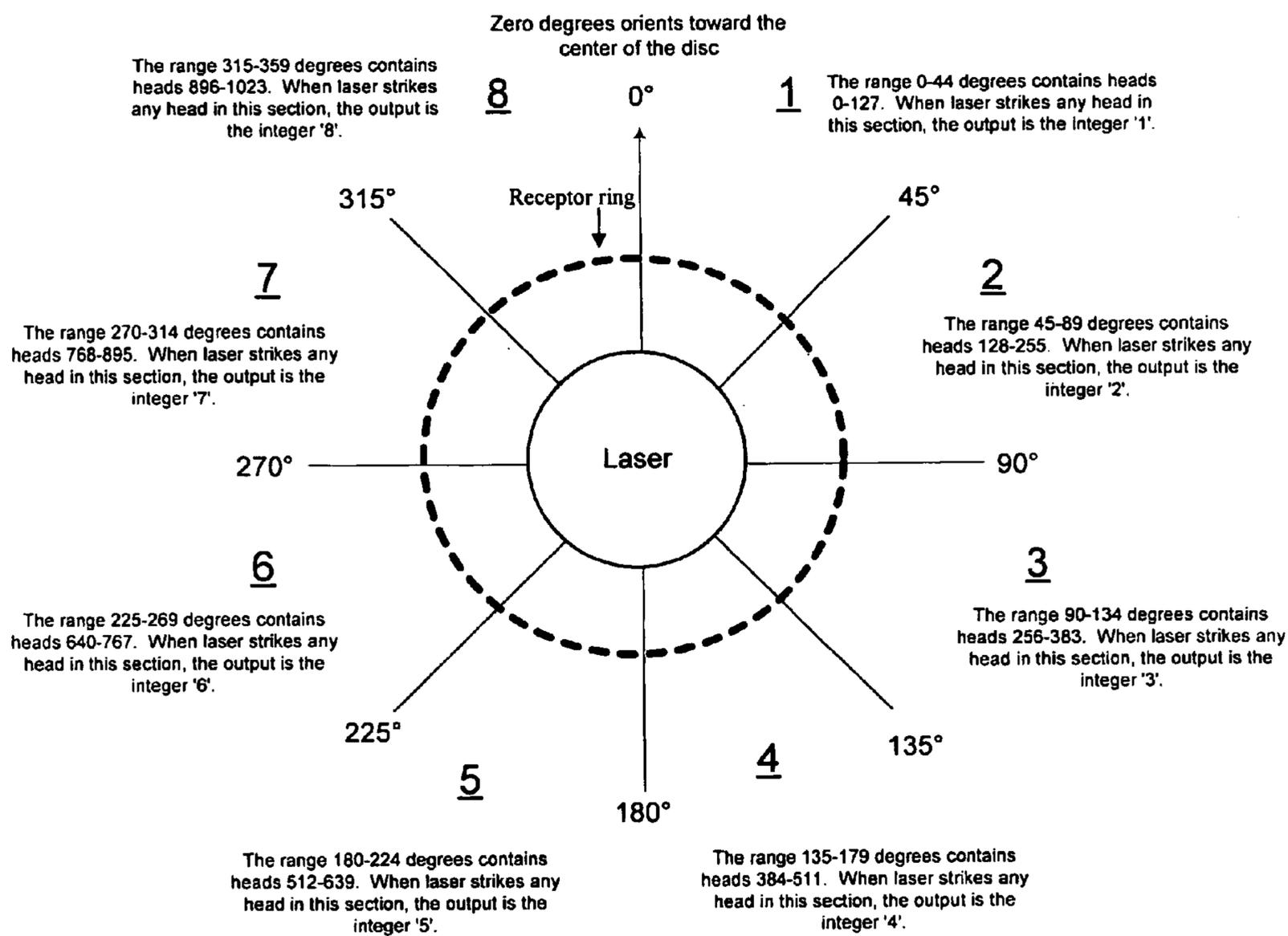
Laser light reflected from a pad on the DDD surface is reflected to one of the sections above and strikes one of the groups of heads in the receptor ring. The output is integer 'x' (any number between 1 and 8), corresponding to the section struck by the reflected light.
