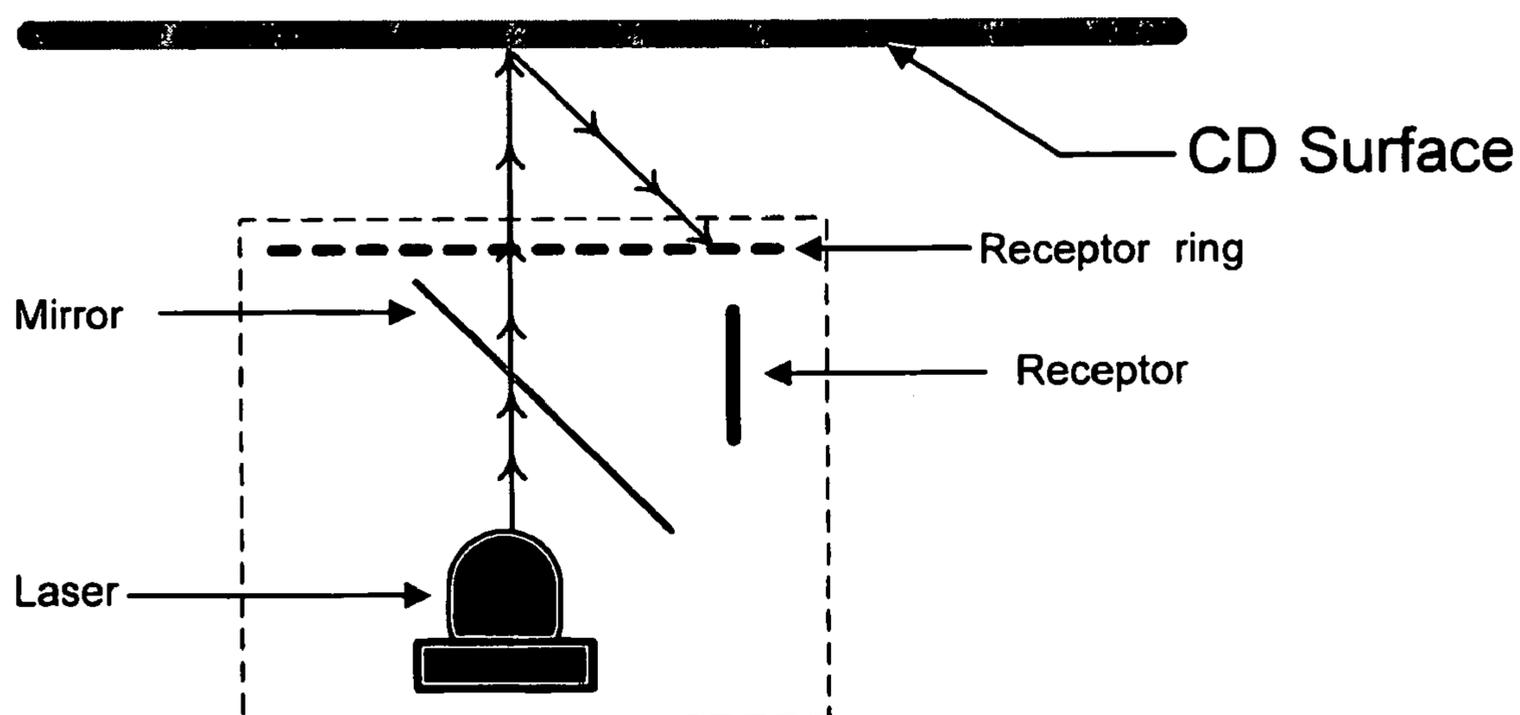
In this diagram, the laser light strikes a pad on the DDD surface and is reflected to one of the heads in the receptor ring. The output is integer 'x' (any number between 1 and 1024), corresponding to the receptor struck by the reflected light.
