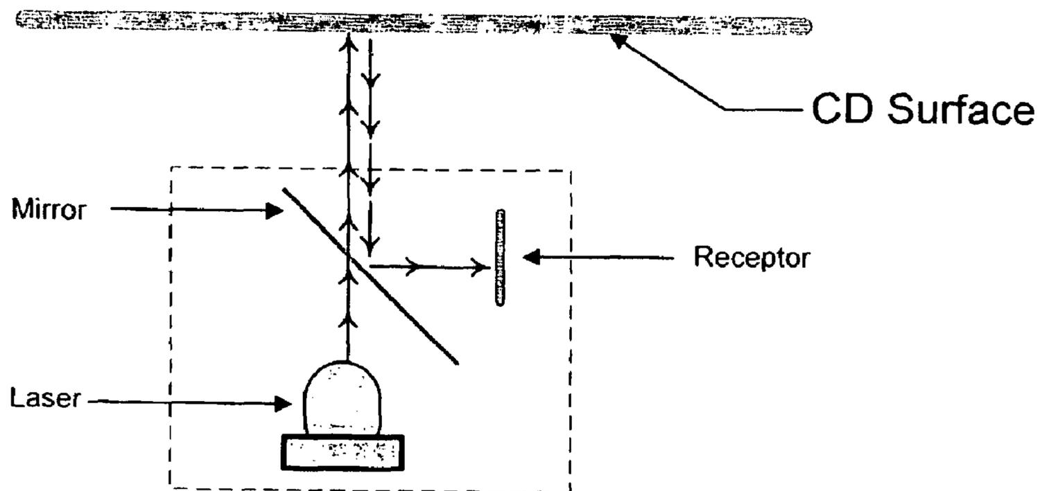
In this diagram, the laser light strikes a stripe on the CD surface and is reflected back toward the laser source. The light is then reflected to the receptor by the mirror and the output is a binary '1'
