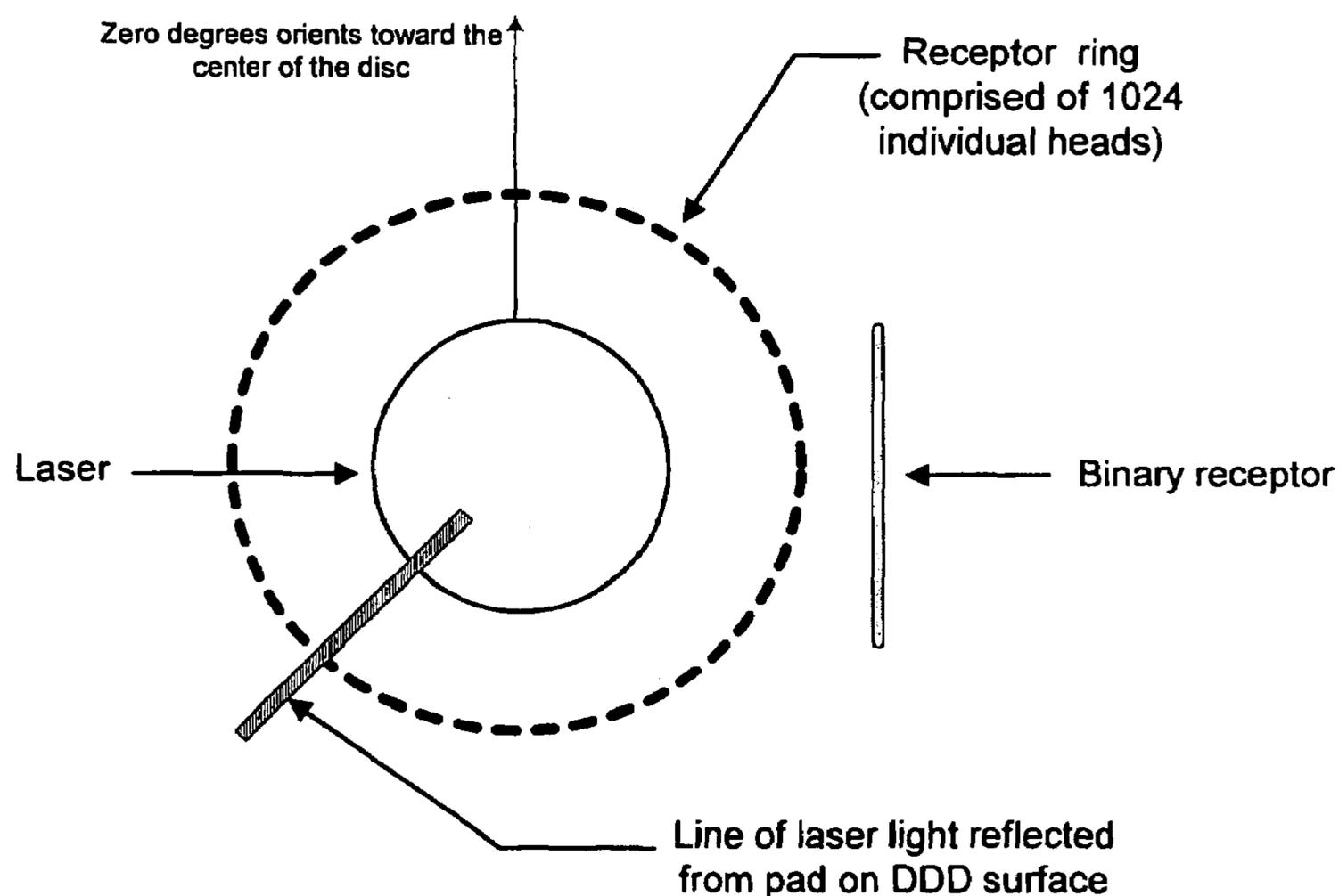
In this diagram, as with diagram 3, the laser light strikes a pad on the DDD surface and is reflected to one of the heads in the receptor ring. The output is integer 'x' (any number between 1 and 1024), corresponding to the receptor struck by the reflected light.
