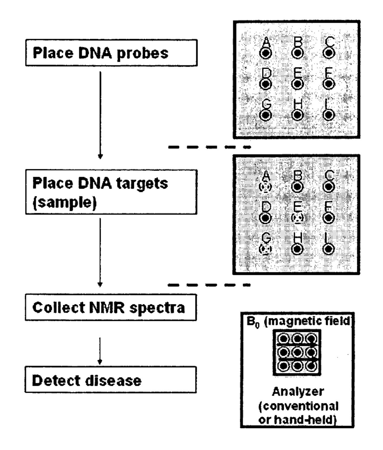
Each letter represents unique DNA probe placed at each NMR microcoil.
