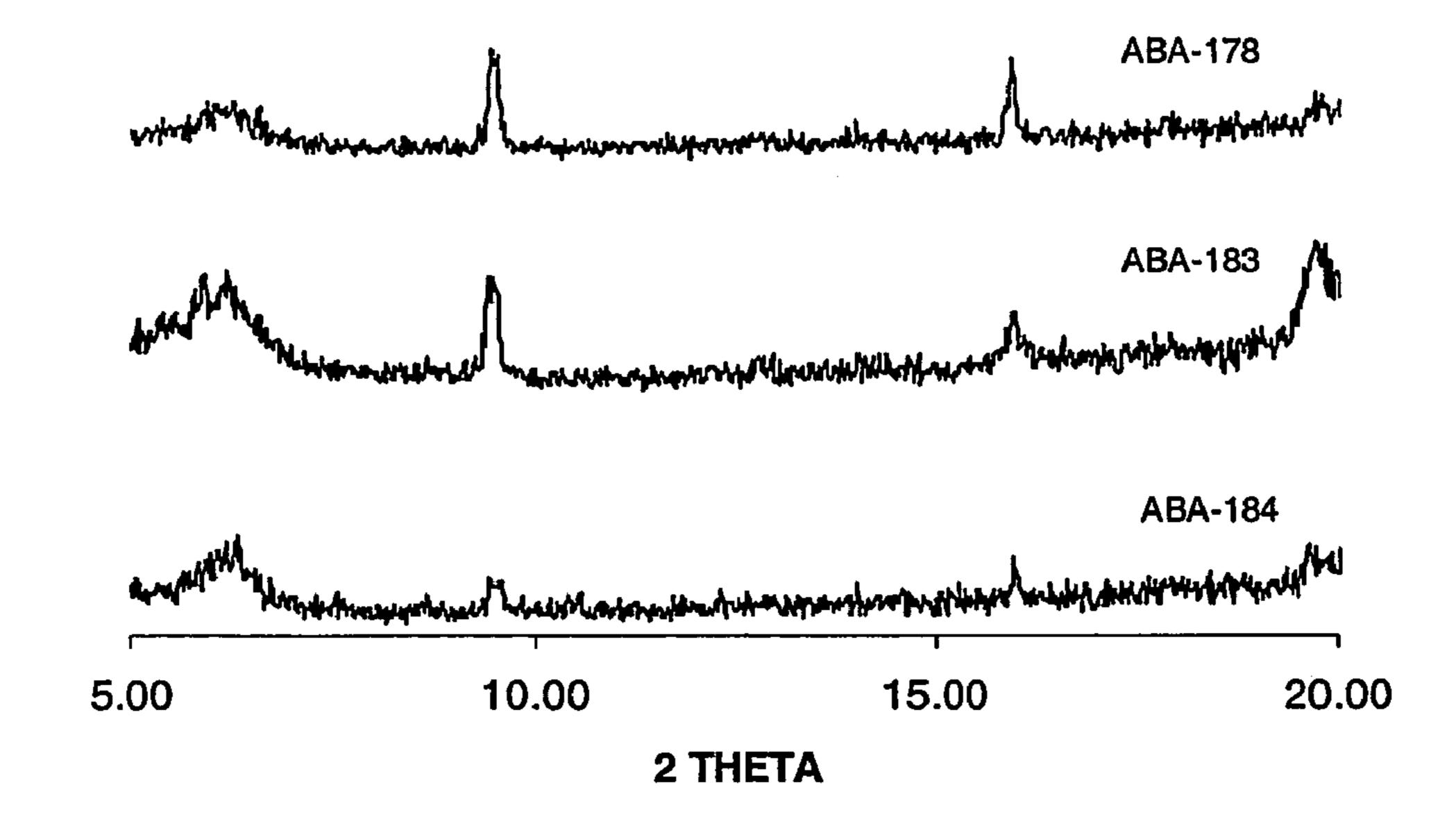
Figure 6 XRD of tablets of alternative binders and AlPO exposed to SAPO-34 synthesis (ABA-178; Example 26 kaoline as binder, ABA-183; Example 27 □-Al<sub>2</sub>O<sub>3</sub> as binder, ABA-184; Example 28 Al<sub>2</sub>O<sub>3</sub>-sol as binder)
