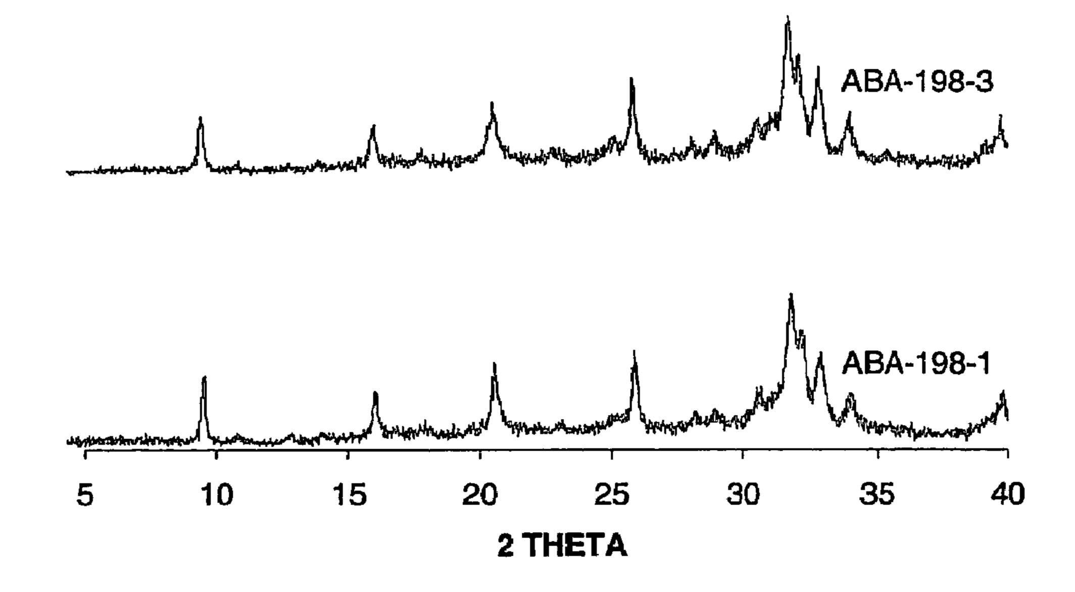
Figure 4 XRD of in-situ synthesis of SAPO-34 in formed bodies (spray dried). The samples were not washed after crystallisation (Examples 20 and 21).
