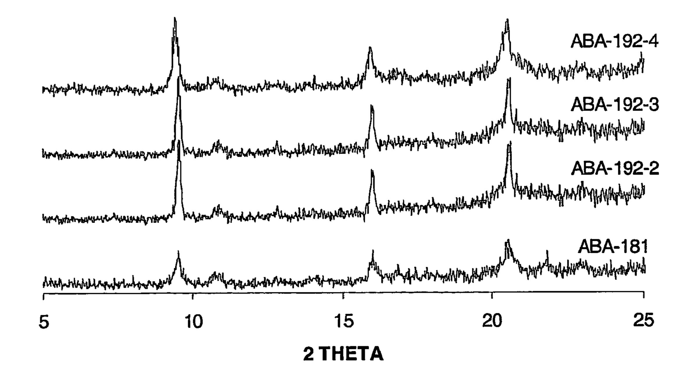
Figure 5 XRD diffractograms of formed bodies after SAPO-34 synthesis (ABA-192-2 (Example 22), ABA-192-3 (Example 23), ABA-192-4 (Example 24) and ABA-181 (Example 25)
