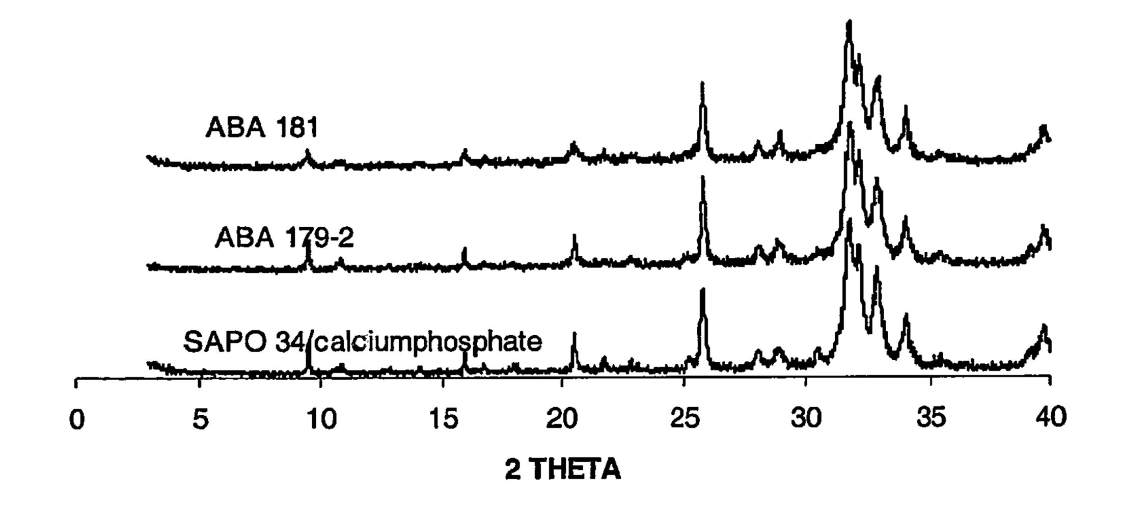
Figure 1 XRD diffractograms of formed bodies after SAPO-34 synthesis (ABA-181; Example 10 and ABA-179-2; Example 1) compared with standard SAPO-34 mixed with calciumphosphate
