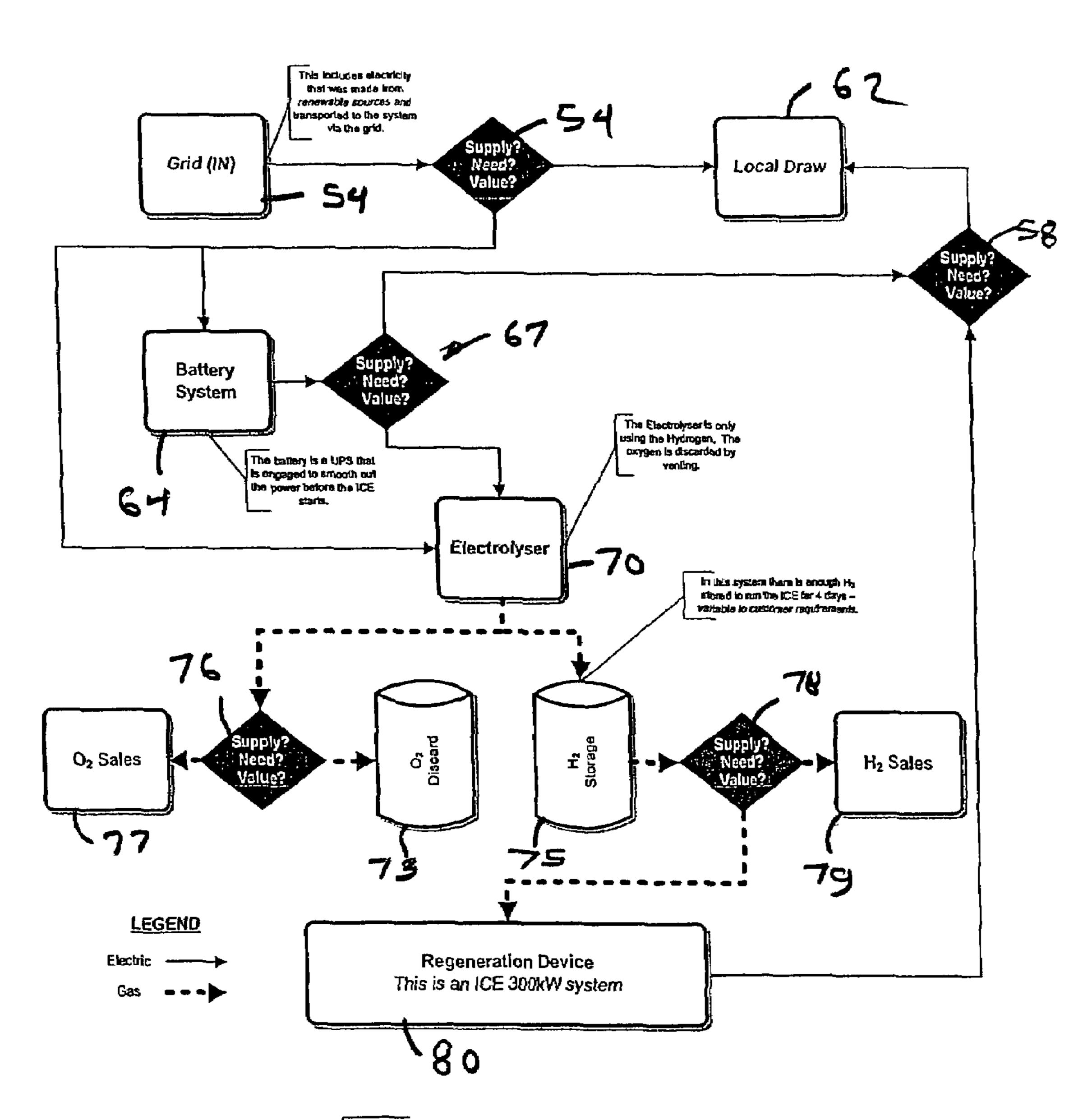
This system is an emergency power system. It is primarily used to provide power when the grid cannot. It can, however, provide ongoing revenue to pay for the equipment for sales of Hydrogen for H<sub>2</sub> vehicle fuel. The Hydrogen is continuously replenished; therefore the system is always ready in case of a power failure.
