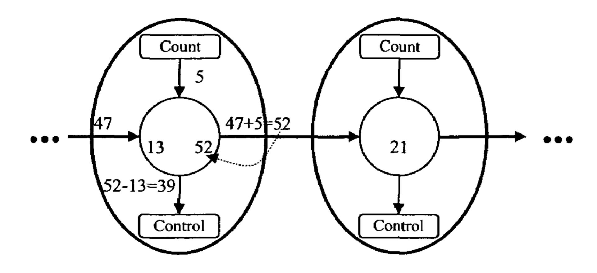
An example of an overflow situation while the system power number is circulating in the ring.
