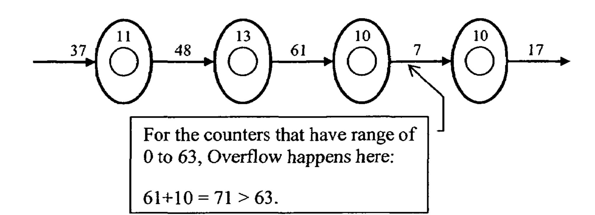
An example of the solution of the overflow situation of the system power number in the ring.
