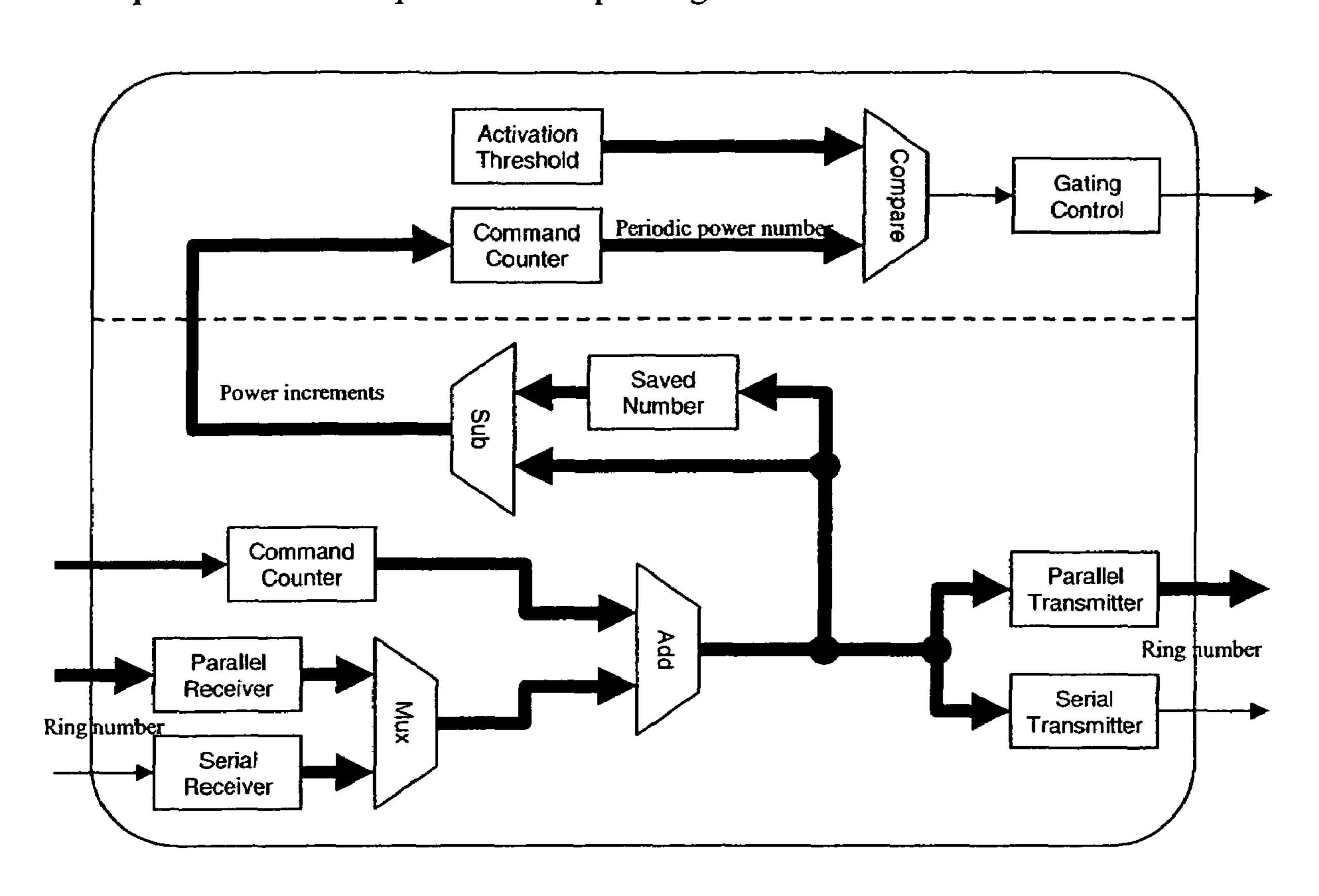
FIGURE 5 An implementation example of ring connections between the power governors
