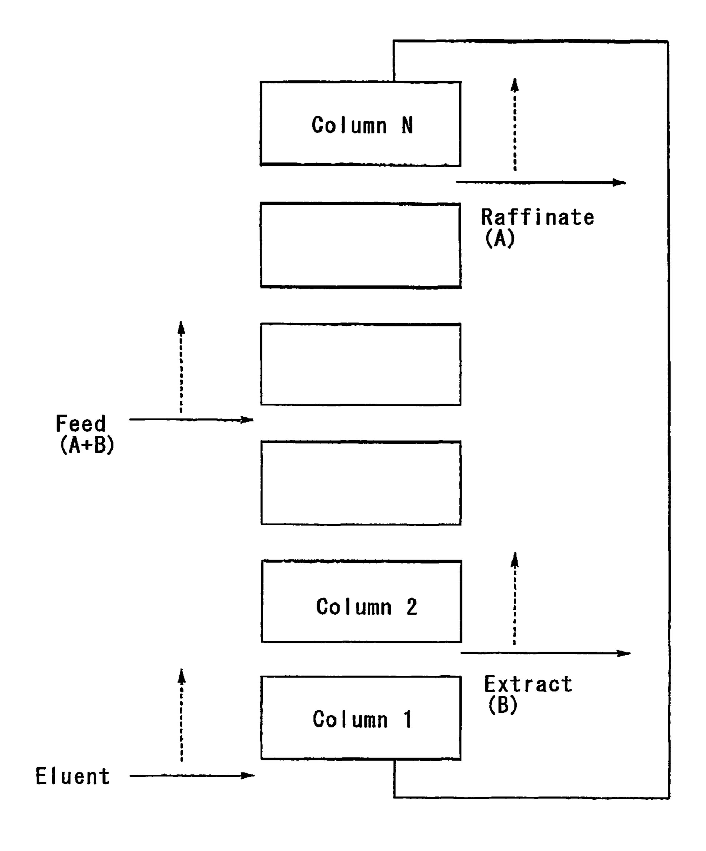
Concept of Simulated Moving Bed (SMB)
