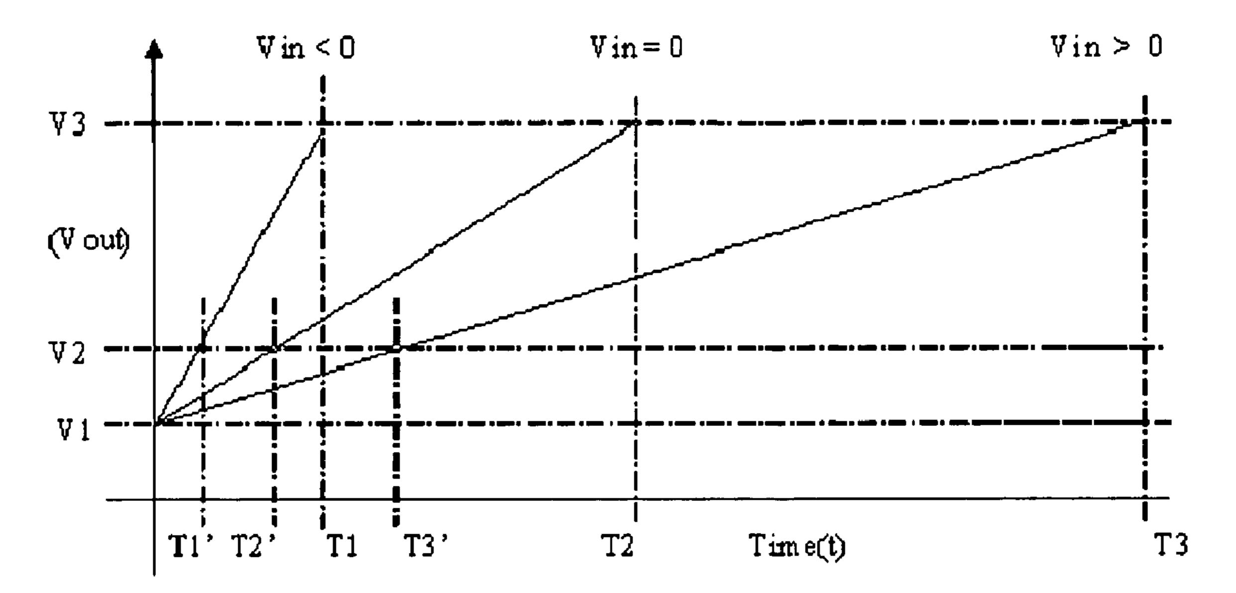
Here Tm1: for Vin < 0, Tm2: for Vin = 0 and Tm3: for Vin > 0 (Where Tin1 < Tin2 < Tin3)
