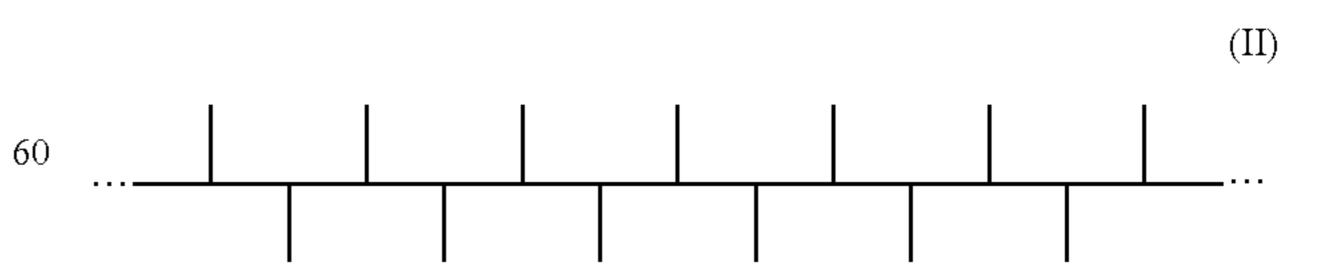
A polymer chain showing no regular order of repeating unit configurations is an atactic polymer. In commercial applications, a certain percentage of atactic polymer is typically
