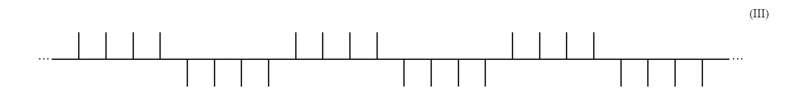
This latter type, the stereoblock polymer, has been success- 15 fully produced with metallocene catalysts as described in U.S. Pat. No. 4,522,982.
